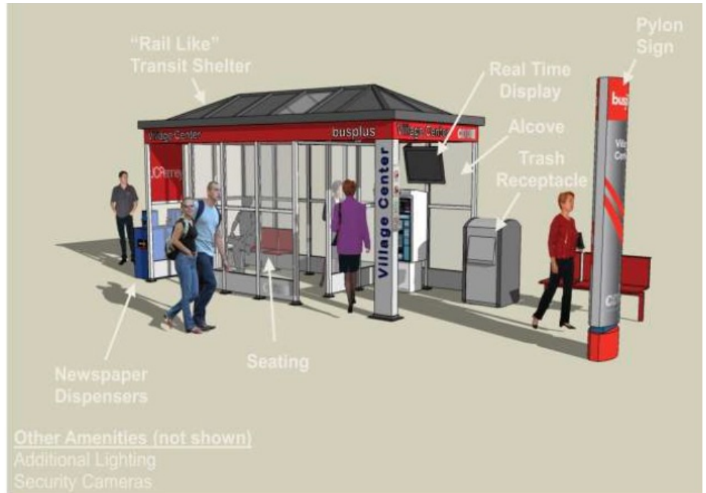
Figure D-4 BusPlus station design, Capital District Transportation Authority (CDTA), Albany, NY
