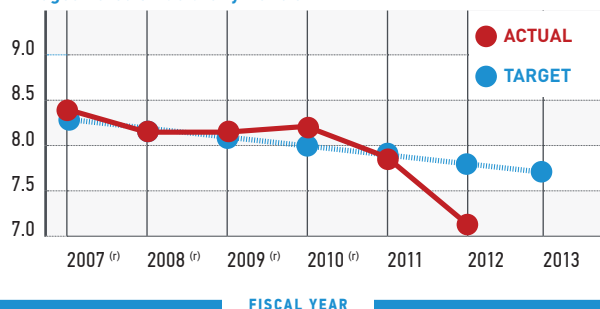
1.2 Percent of Deck Area (i.e., the Roadway Surface of a Bridge) on NHS Bridges Rated Structurally Deficient
