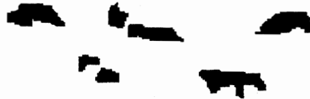
Figure 3.8 Binary representation of Figure 3.7 after thresholding at a level of 56.
