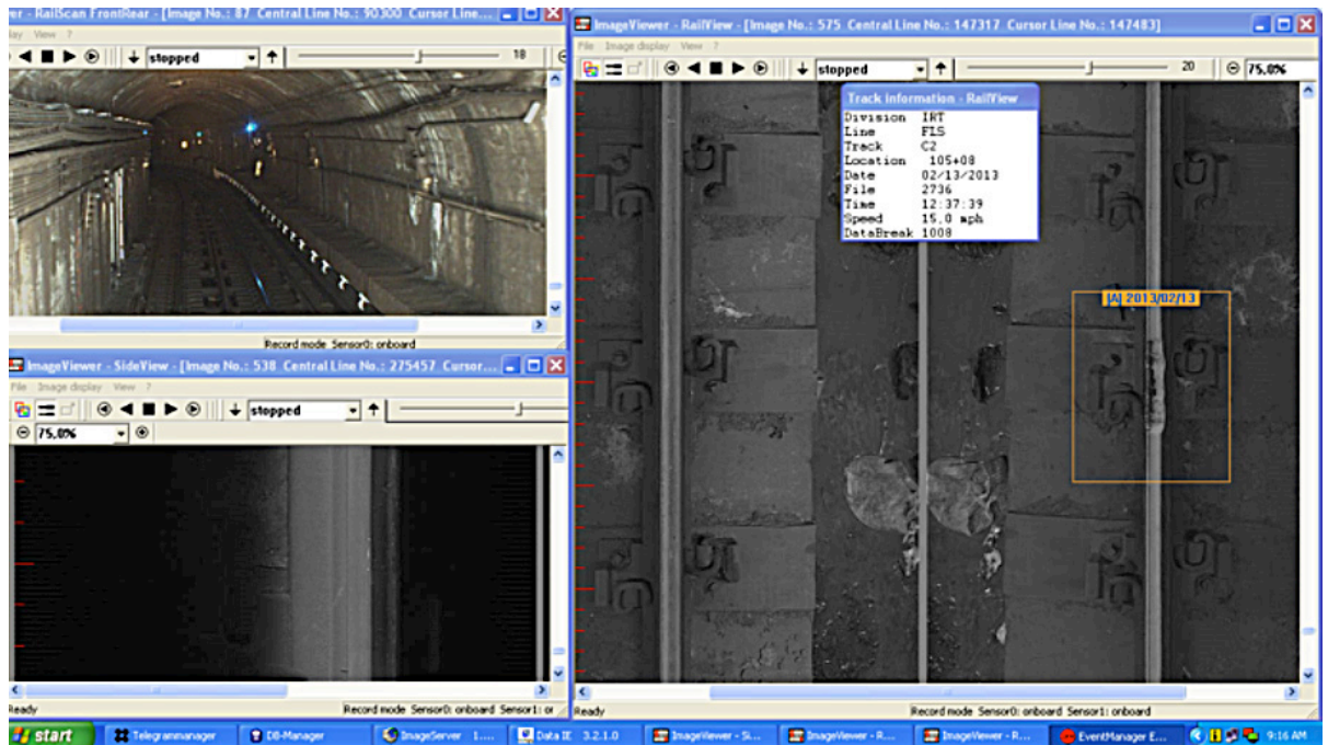
Figure 4-36 Same Rail View defect detected and marked in 2/13/2013 inspection run
