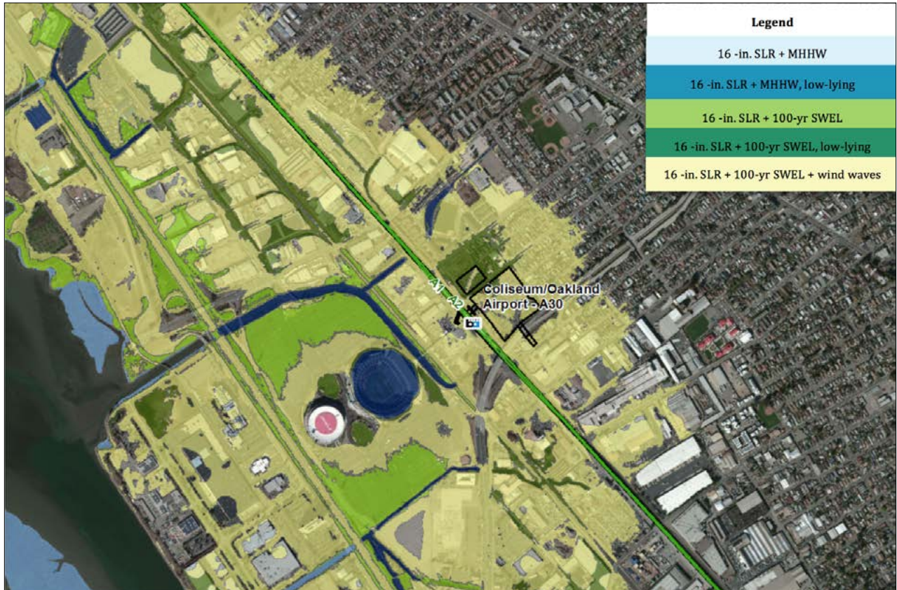
Figure 3-16 Sea-Level Rise Scenarios in 2050 near Oakland Coliseum Traction Power Substation
