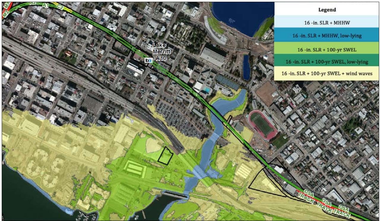
Figure 3-5 Sea-Level Rise Scenarios in 2050 near Lake Merritt Station Entrance
