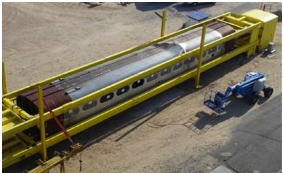
Figure 7-4 Passenger car structural test facility at TTC
