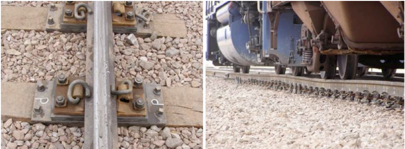
Figure B-12 Adjustable tie plates for vertical and lateral track geometry perturbations
