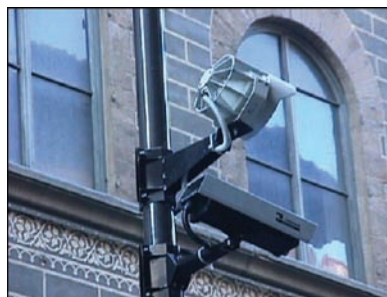
Typical ALPR camera and illumination device.
