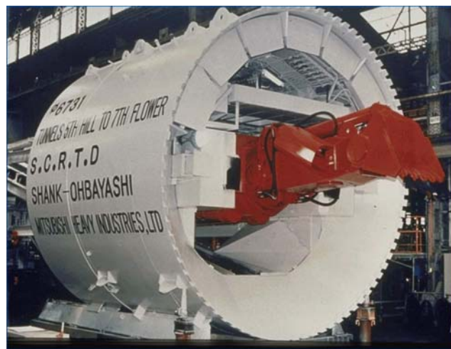
Figure 7-2 Digger Shield with Hydraulically Operated Breasting Plates on Periphery of Top Heading of Shield used to Construct Transit Tunnel.
