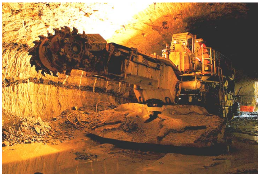
Figure 6-16 AM 105 Roadheader, Australia
