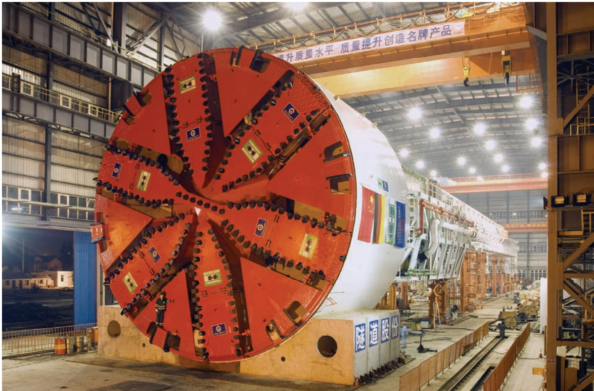
Figure D-13 Photograph of Herrenknecht S-317 Mixshield TBM
