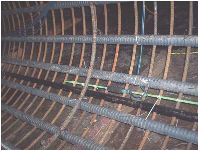
Figure 68. Photo. Coupled VW (blue cable) and RT (green cable) gauges.
