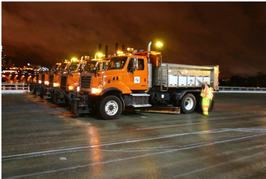
Figure 98. Photo. Trucks (400-kip (181,436.95-kg) total load) staged at predetermined location.
