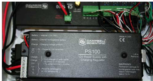
Figure 37. Photo. Campbell Scientific, Inc.® PS100 12-V power supply with rechargeable battery.
