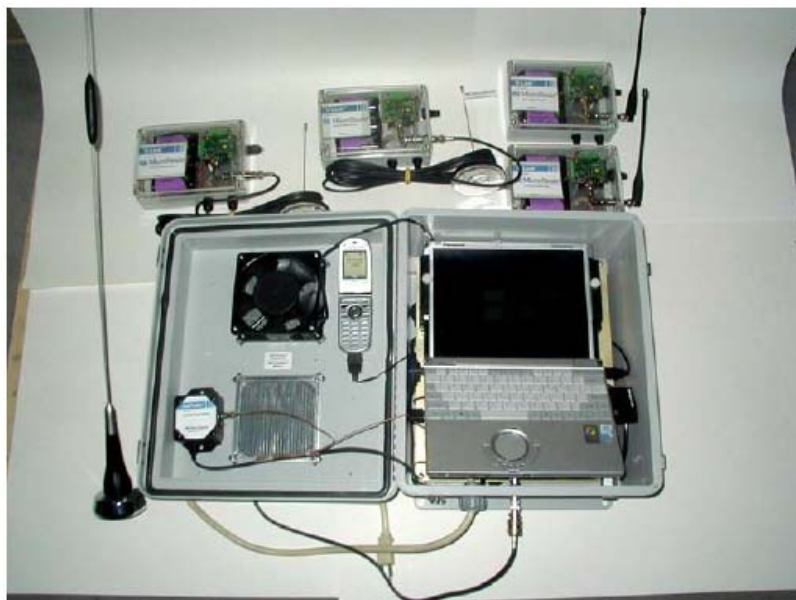
Figure 8. Photo. Wireless data collection and transmit setup. (2)
