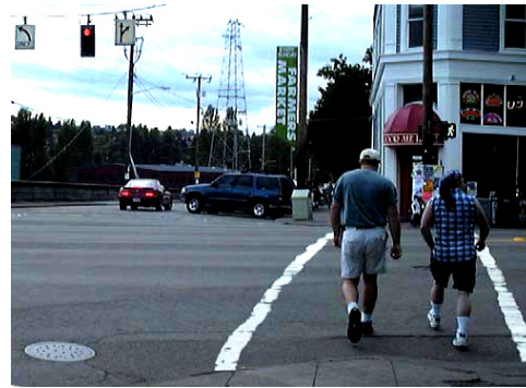
Figure B. With a leading pedestrian interval, pedestrians get an advance walk signal before motorists get a green. This gives the pedestrians several seconds to establish their presence in the crosswalk before motorists start to turn.
