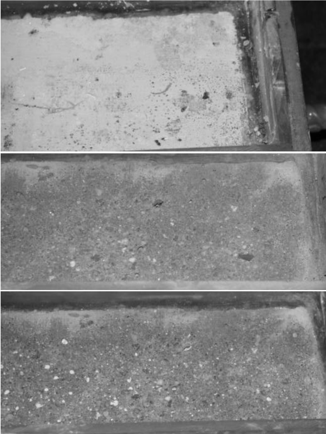
Figure 25. Type I specimen surface appearance: (Top) after ECE but prior to sandblasting, (Middle) after sandblasting but prior to second application of ECE, (Bottom) following a second application of ECE for 12 hours
