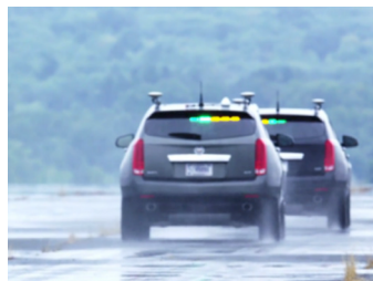
The green and yellow lights on the test vehicles indicate communication and connectivity between the cars.
