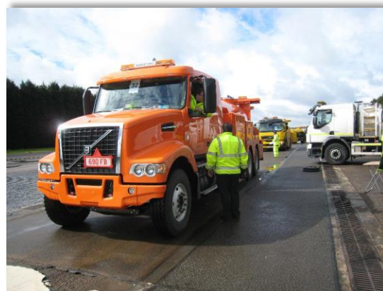
FHWA's orange Sideway-force Coefficient Routine Investigation Machine
