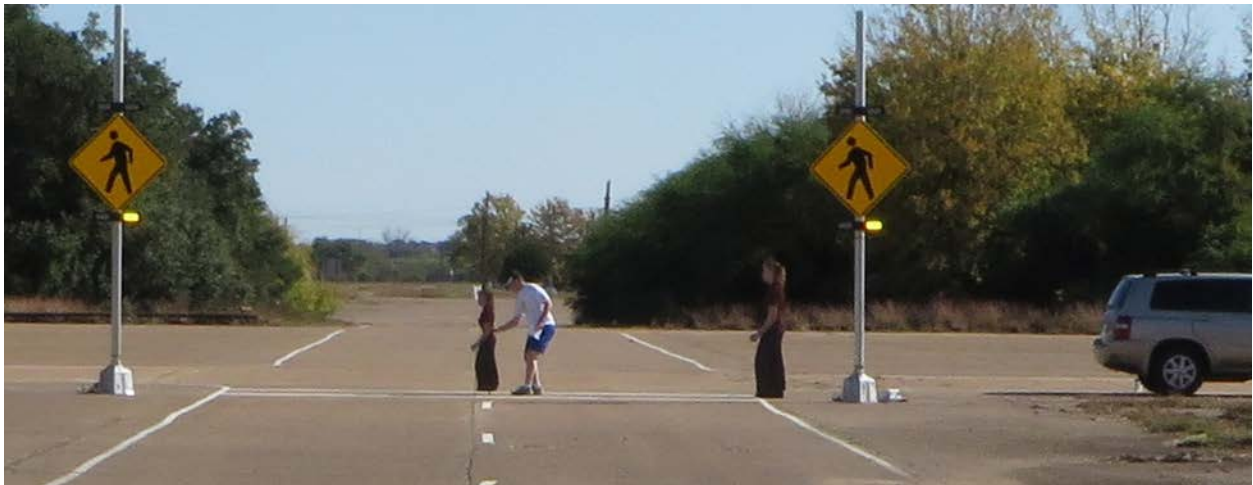
Figure 7. Photo. Researcher removing short cutout pedestrian after placing tall cutout pedestrian.
