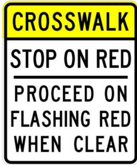
Figure 58. Photo. Sign recommended by FHWA to address comprehension issues with the flashing red phase.
