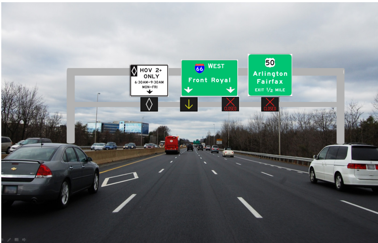
Figure 29. Photo. Picture shown for the two right lanes closed scenario for the Minnesota-based signs.
