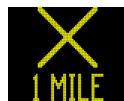
Figure 45. Graphic. Lane closed ahead with legend option used in first simulator study.
