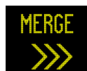
Figure 46. Graphic. Merge right with legend option used in first simulator study with streaming chevrons).
