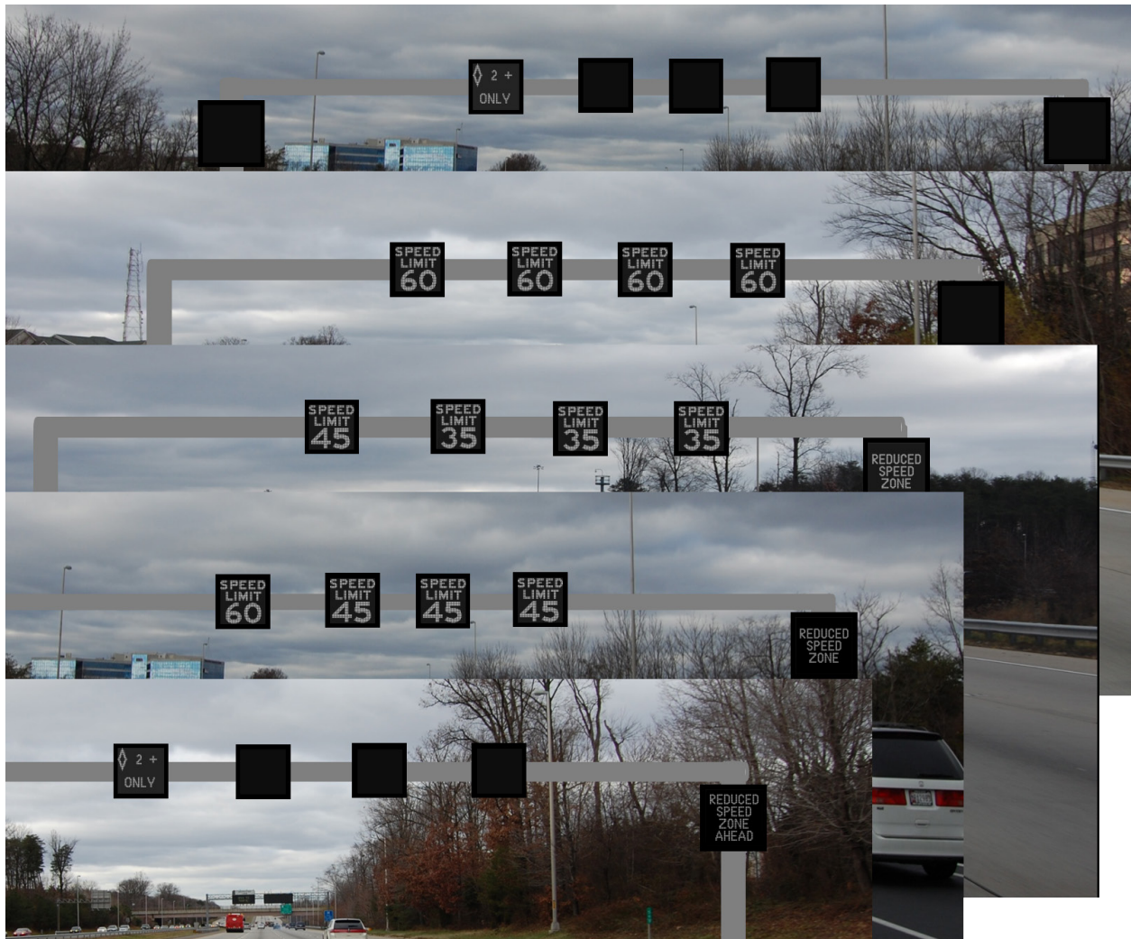
Figure 2. Screen capture. VSL scenario that shows the progression of what a driver would see driving down the road, going from bottom to top.
