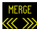
Figure 48. Graphic. Merge left or right with legend option used in first simulator study with chevrons streaming.
