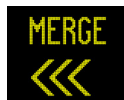
Figure 47. Graphic. Merge left with legend option used in first simulator study with chevrons streaming.
