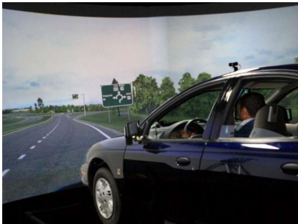
Figure 42. Photo. The FHWA Highway Driving Simulator.
