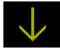
Figure 5. Graphic. Flashing or static lane open with caution sign adapted from Minnesota deployment.
