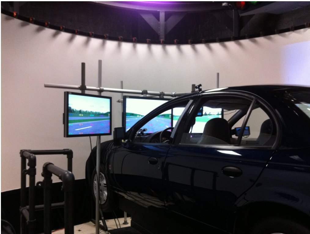
Figure 77. Photo. The FHWA Highway Driving Simulator with LCD monitors.
