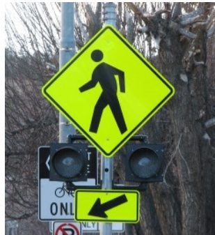
Figure 85. Photo. Circular beacons used at FG-01.
