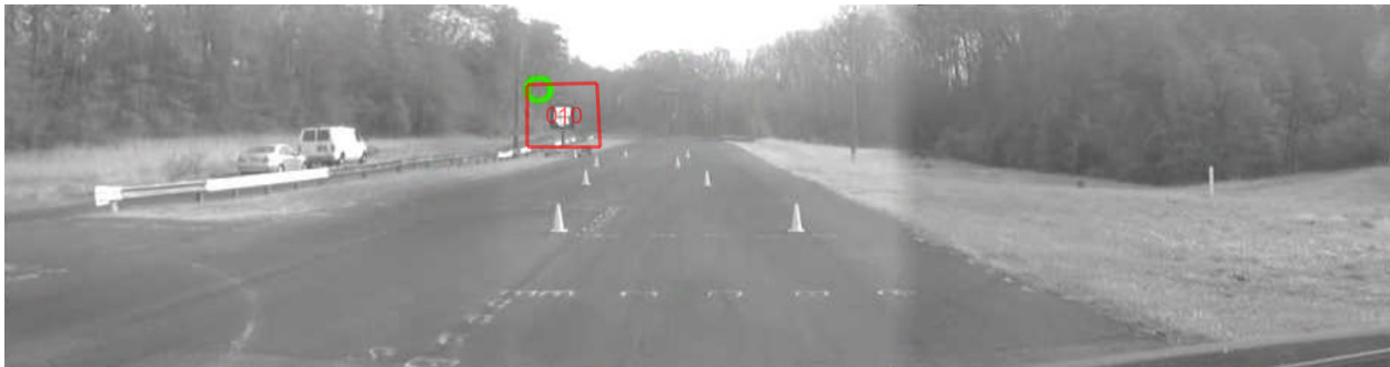
Figure 25. Screen capture. Two-degree ROI for the CMS approximately halfway down the slalom course.
