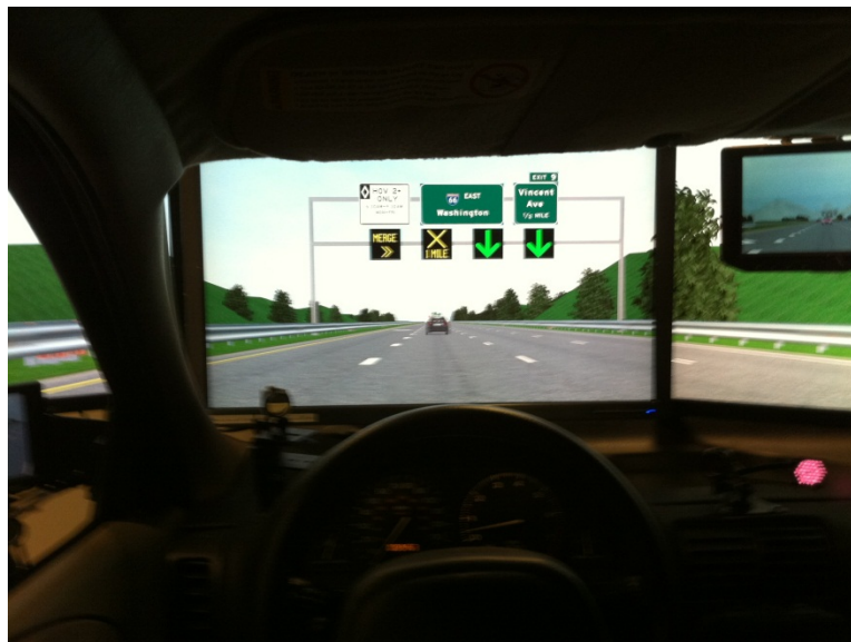
Figure 55. Photo. View of the three LCD monitors from slightly behind the driver's eye point.
