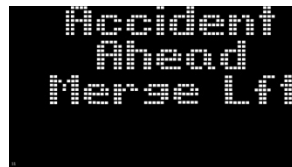
Figure 10. Photo. Accident ahead merge left sign with white pixels that yielded a mean similarity rating of 5.6 between the CMS and LCD displays.
