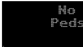
Figure 14. Photo. No peds message on LCD with emulated CMS pixels.
