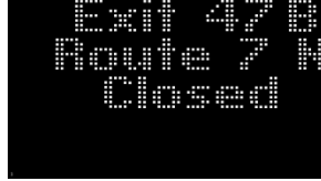
Figure 16. Photo. Exit 47 B message on LCD with emulated CMS pixels.
