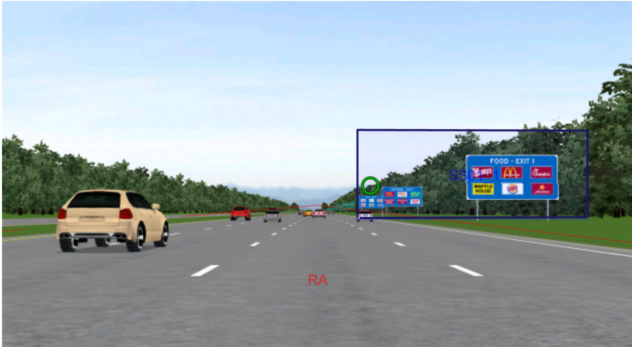
Figure 56. Screen capture. Analyst's screen for coding shows ROI for specific-service signs that are 400 ft (122 m) apart.
