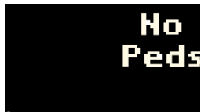
Figure 15. Photo. No peds message on LCD with filled-in space between emulated CMS pixels.
