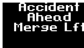
Figure 12. Photo. Accident ahead merge left sign with solid white letters that yielded a mean similarity rating of 5.6 between the CMS and the LCD displays.
