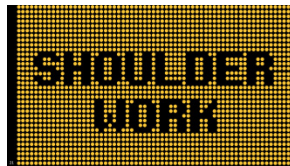
Figure 18. Photo. Shoulder work CMS message emulation on LCD.
