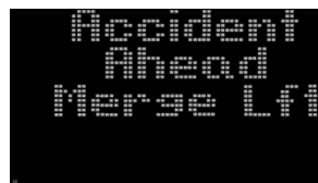
Figure 11. Photo. Accident ahead merge left sign with grey pixels that yielded a mean similarity rating of 4.7 between the CMS and LCD displays.
