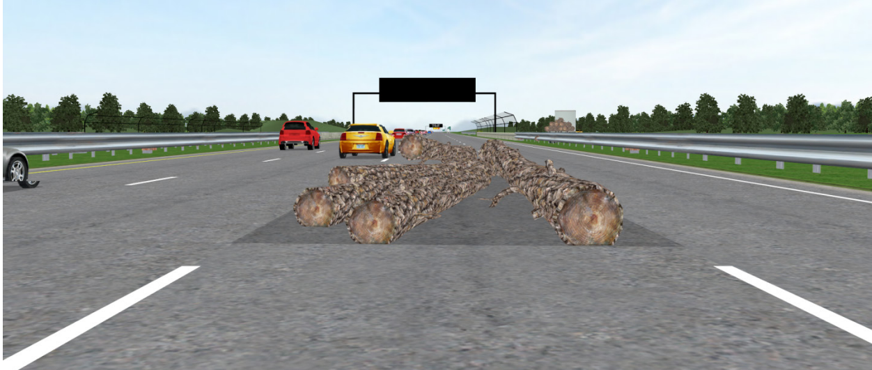
Figure 42. Screen capture. Driver's view of spilled load from 128 ft (39 m).
