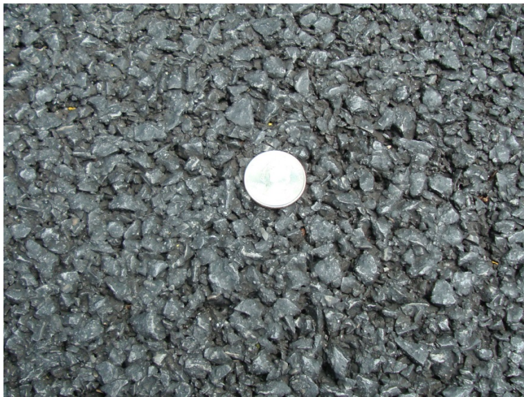
Figure 7. Placement of an UTBWC using a self-priming paver (top) and surface texture of an UTBWC (bottom). (34)
