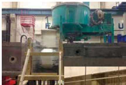
Casting of beam splice connection.
