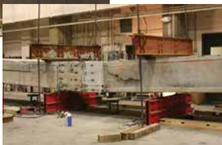
Full-scale flexural test of a beam splice connection made of Ultra-High Performance Concrete.
