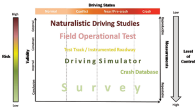
The relationship between research methods and impacting factors. Note: There are five empirical factors that can be used to evaluate the quality of data and the analysis performed. The five factors are: driving states, risk, level of control, measurements, and validity. The five factors presented in this figure explain the similarities, differences, advantages, and disadvantages among the different research methods.
