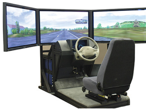
Figure 4. The National Advanced Driving Simulator miniSim Simulator.
