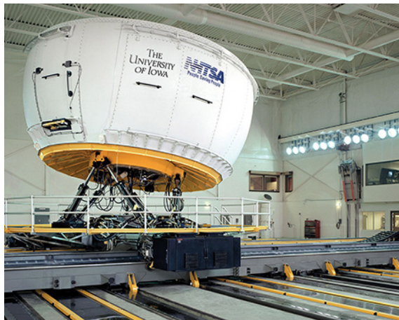
Figure 1. The National Advanced Driving Simulator motion-base driving simulator.
