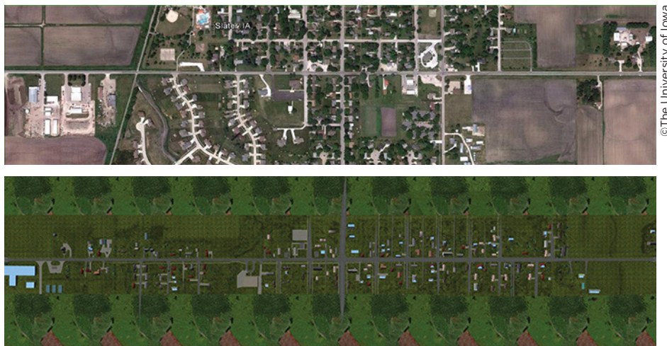
Figure 5. Example of geometric matching of real (top) and simulated (bottom) roadway geometry of a gateway in Iowa.
