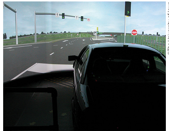
Figure 2. The Federal Highway Administration motion-base driving simulator.
