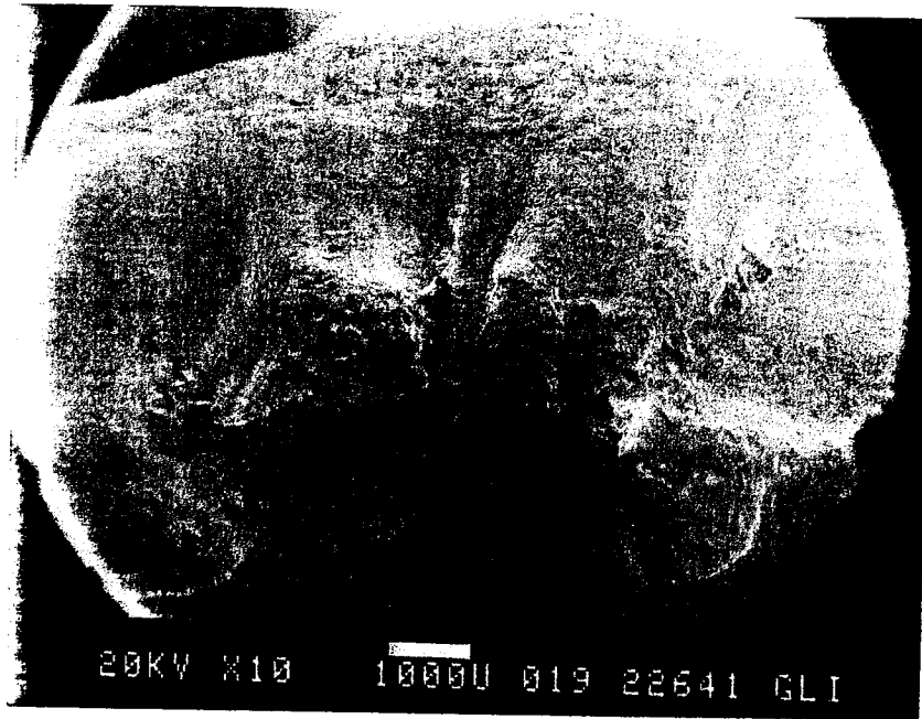
Figure 21. Overview of weld fracture on Sample SEM 3.
