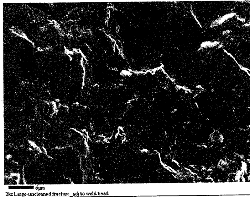
Figure 18. SEM photomicrograph showing intergranular fracture observed adjacent the reference upstream girth weld in the lack of fusion / fatigue zone transition. 2000X magnification.
