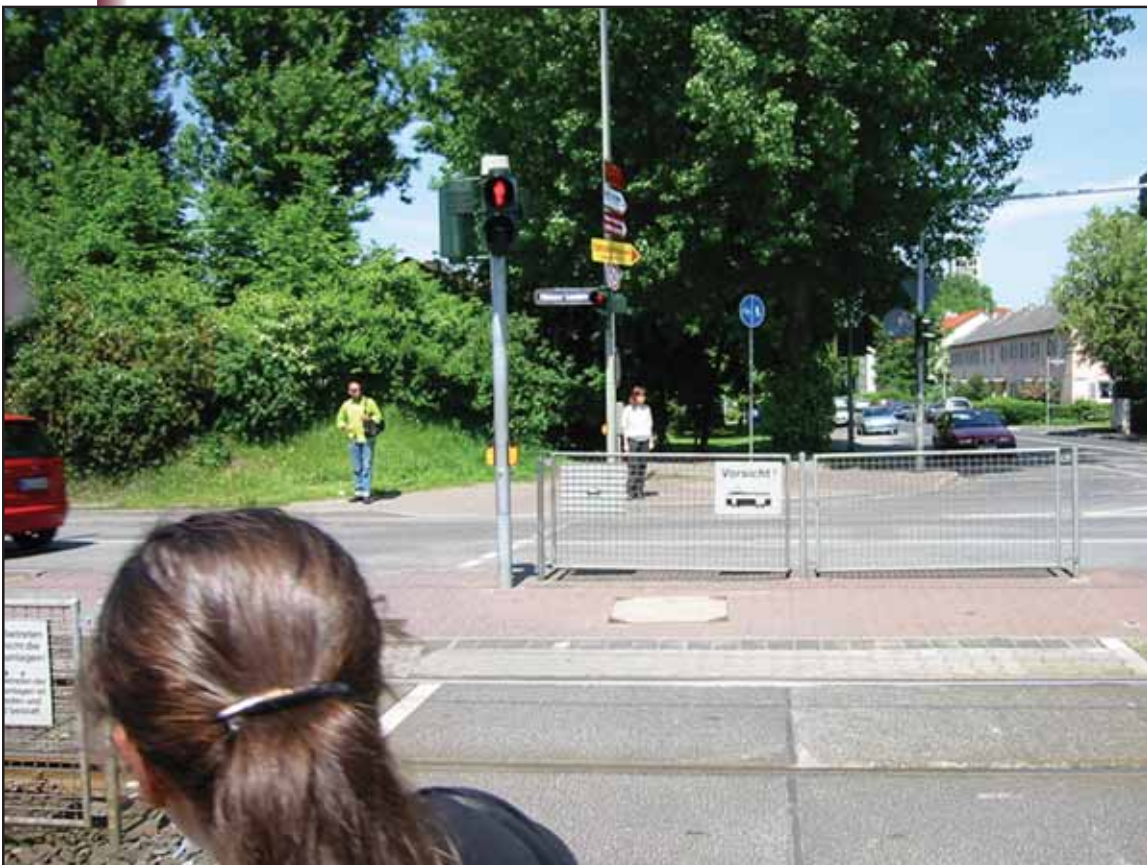
Figure 5-2. Staggered pedestrian crossing in Germany.
