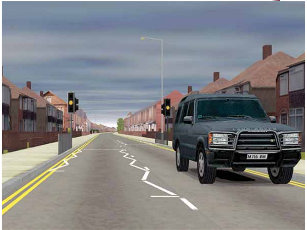
Figure 2-5. Vehicle simulator to test extended amber timing in the United Kingdom.
