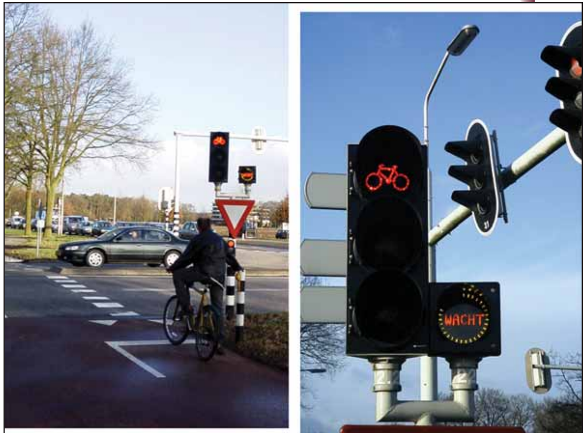
Figure 4-20. Countdown indicator for bicycle crossing.
