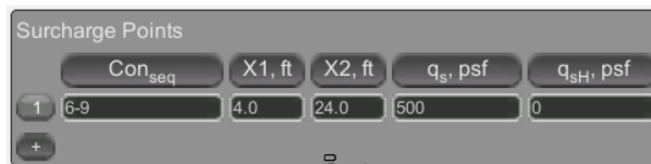
Figure 50. Screen Shot. Surcharge location and magnitude
