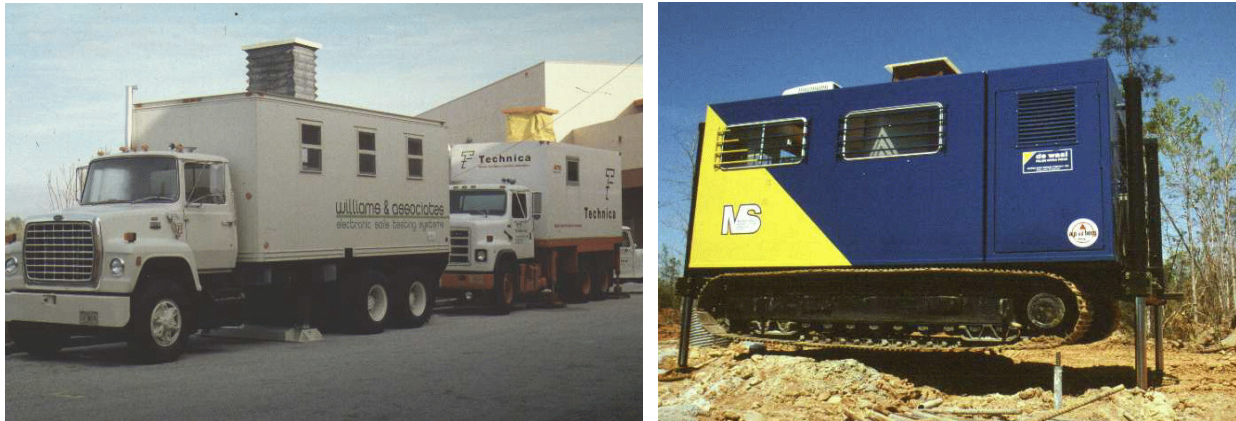
Figure 5-2. Direct-Push Technology: (a) Truck-Mounted and (b) Track-Mounted Cone Rigs.
