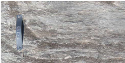
Figure 5: Cross checking of juvenile wood in Southern Catalpa after 12 months of weathering in WI.
