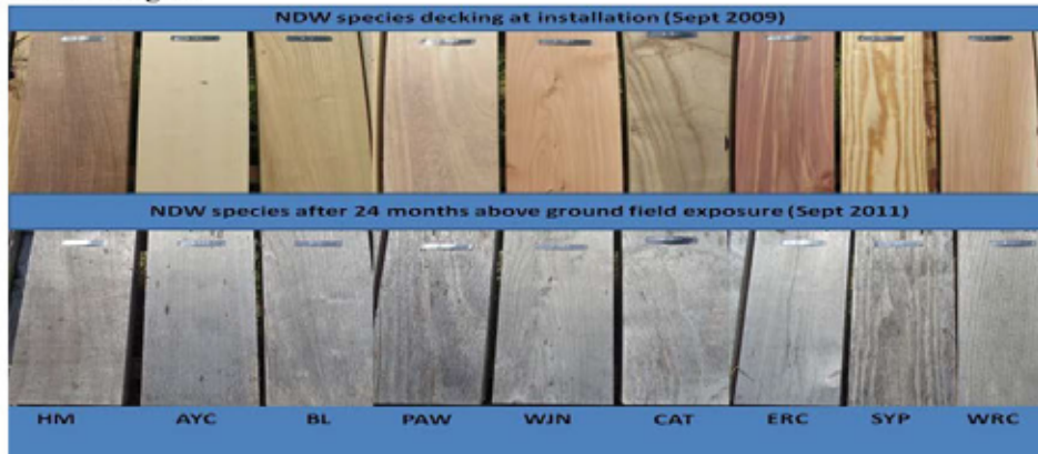
Figure 3: Composite image showing NDW decking specimens at installation (top) compared to NDW specimens after 24 months above ground field exposure (bottom). (HM=honey mesquite, AYC=alaska yellow cedar, BL=black locust, PAW=paulownia, WCJ=west coast juniper, CAT=southern catalpa, ERC=eastern red cedar, SYP=southern yellow pine (control), and WRC= western red cedar.)
