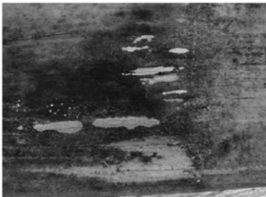
Figure 7: Incipient decay by white rot fungi noted on the underside of SYP decking specimens after 12 months field exposure in WI.
