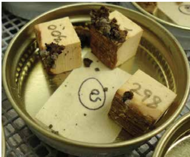
Figure 24. Unextracted blocks of AYC after 8 wk of soil bottle exposure to G. trabeum . Note localized patterns of brown-rot only on the underside of block that abutted the feeder strip.
