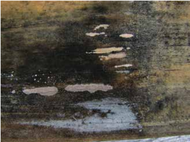
Figure 11. After 12 months outdoor exposure in Wisconsin (Decay hazard zone 2) the underside of the Southern Pine controls with fruiting bodies present and stringy bleached undersides, indicating colonization by white-rot fungi along with black mold.
