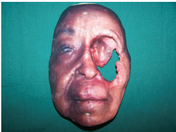
Figure 5 Color model made with the ZPrinter ® 450 and high performance composite material.
