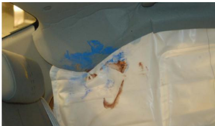
Figure A-74: Post-Test Rear Passenger Dummy Close-Up Head Contact with Side Airbag View
