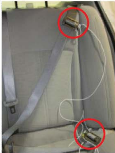
Lap and Shoulder load cells – forces on belts
