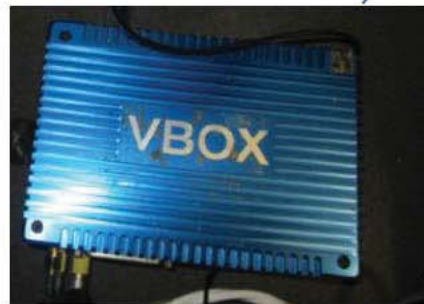
VBOX – provides velocity data from GPS.
