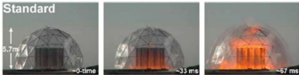
Figure 38: High-speed optical video images of hydrogen combustion for a 30% hydrogen/air mixture, ignited with a 40 J spark. Figure reproduced from Reference [112].
