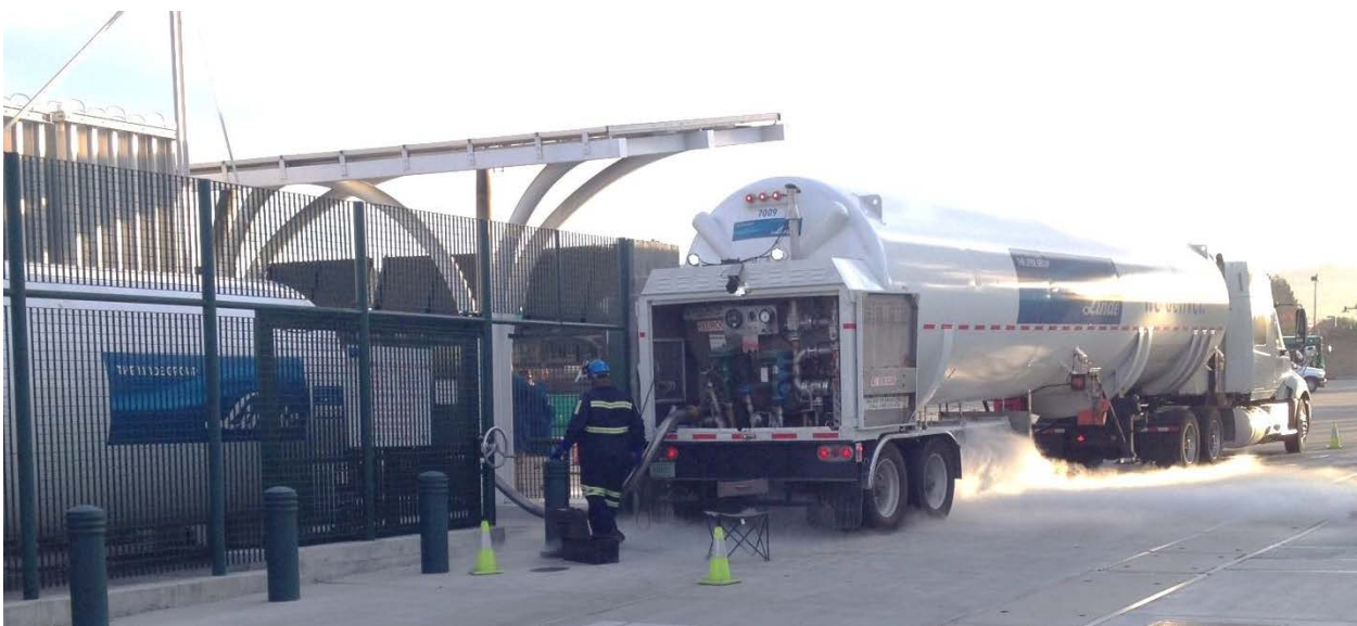
Figure 44: LH 2 transfer operation at AC Transit, Emeryville, CA, performed by Linde.
