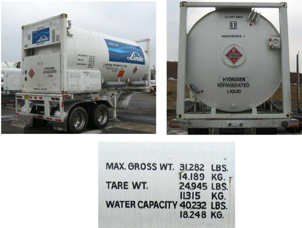
Figure 20: Photographs of a Linde ISO LH 2 container (tank) mounted on a trailer. The rectangular frames on the tank allow for convenient lifting and transport. The specifications written on the side of the tank are shown in the lower picture.
