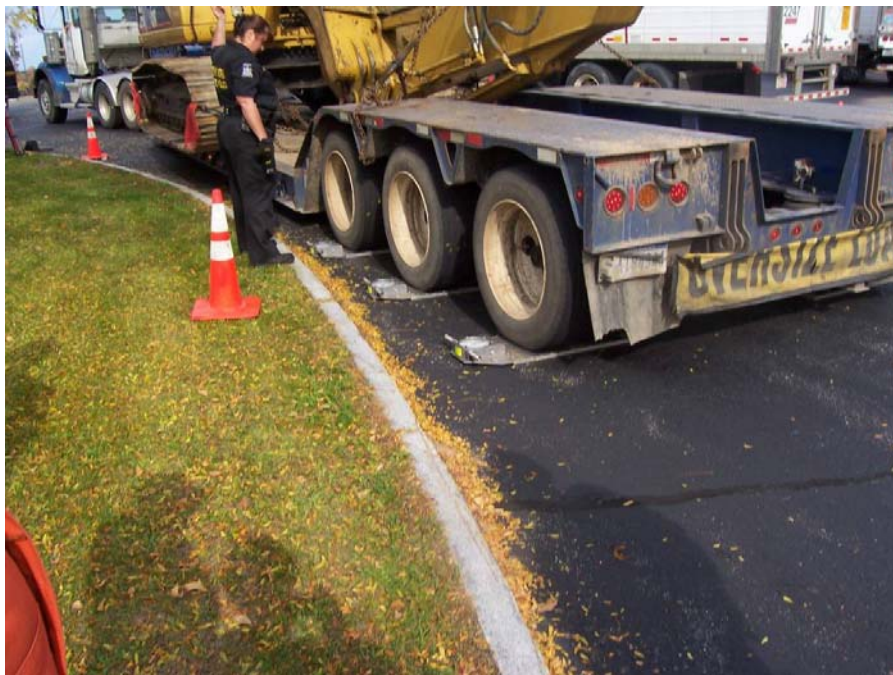
Figure 7-4. Portable Truck Scales in Use at the Schodack Rest Area on Westbound I-90 in New York
