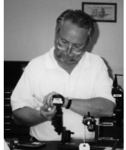
Hill Air Force Base Technician testing a bolt for thread dimensions during OIG's audit of aviation threaded fasteners.
