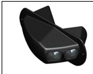
Figure 3. Image. Close-up of BSW sensor housing.
