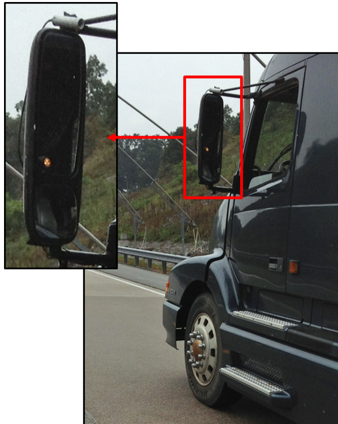
Figure 9. Image. BSW system's visual alert mounted on flat mirror.
