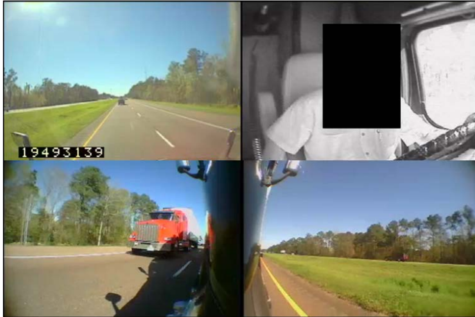
Figure 20. Photo. Four camera images multiplexed into a single image.
