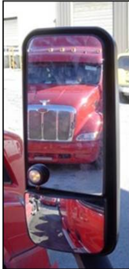
Figure 4. Image. BSW visual warning mounted on CMV flat mirror.
