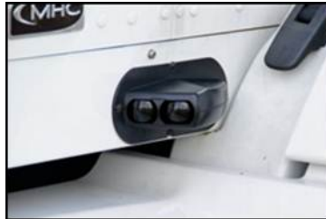
Figure 2. Image. BSW sensor housing installed on tractor-trailer.
