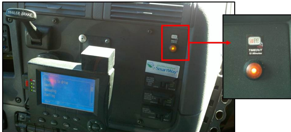
Figure 21. Image. Temporary disengage pushbutton for the BSW system.
