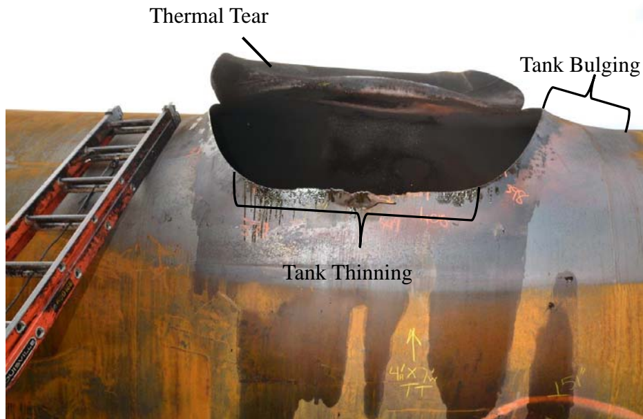
Figure 2. CPC-1232 tank car CBTX 741946 thermal shell tear surrounded by a bulging and thinning shell.
