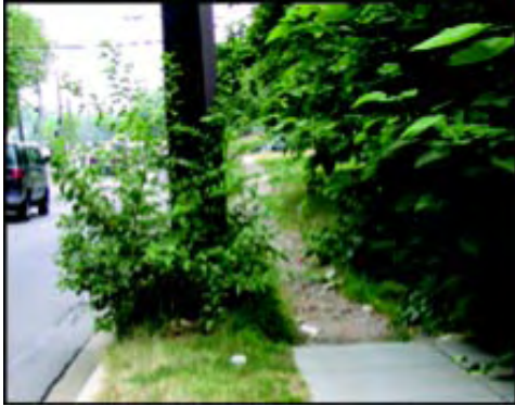
The well-trodden path that continues where the sidewalk ends provides evidence that pedestrians continue to use this route. Designers should look for such clues when considering locations for infrastructure improvements for foot traffic.
