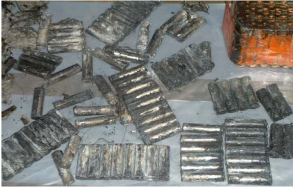
Figure 2. Scorched Lithium Batteries
