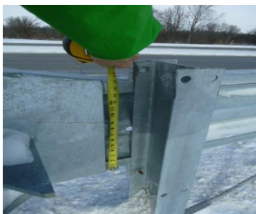
Guide Chute Exit Height (outside)
