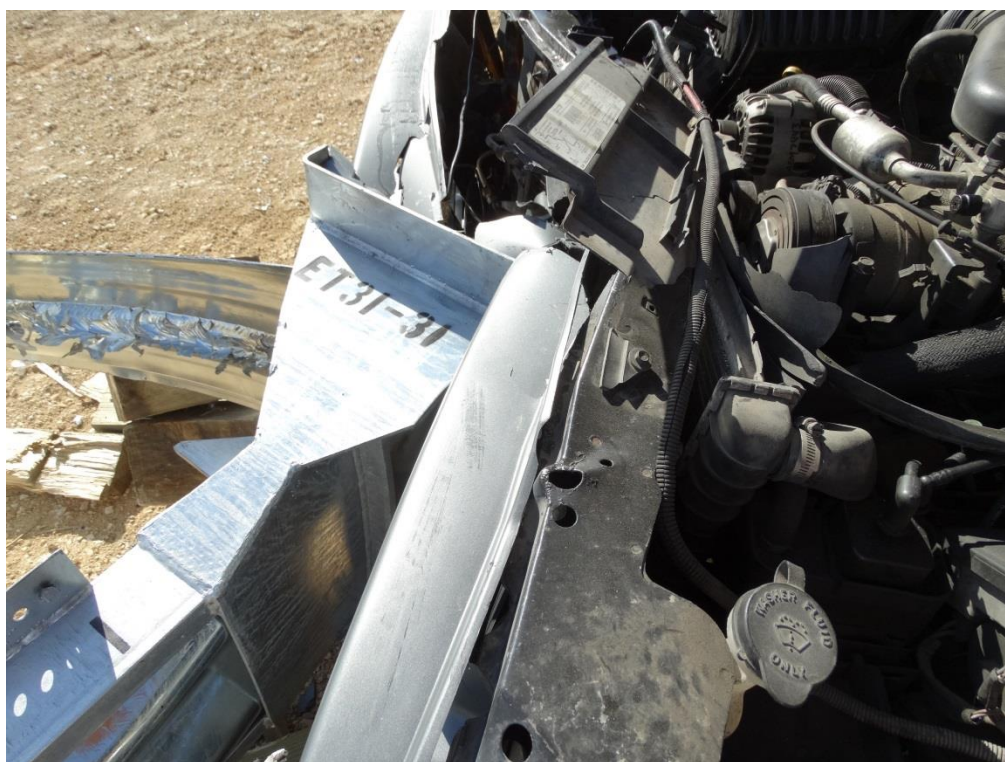
Figure 3.35: Post-Test – ET Plus Head at Front of Vehicle
