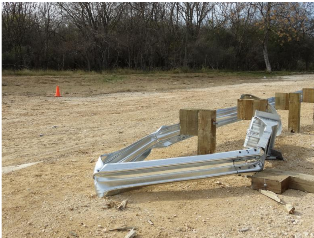
Figure 3.10: Post Test – Side View of Gated Terminal
