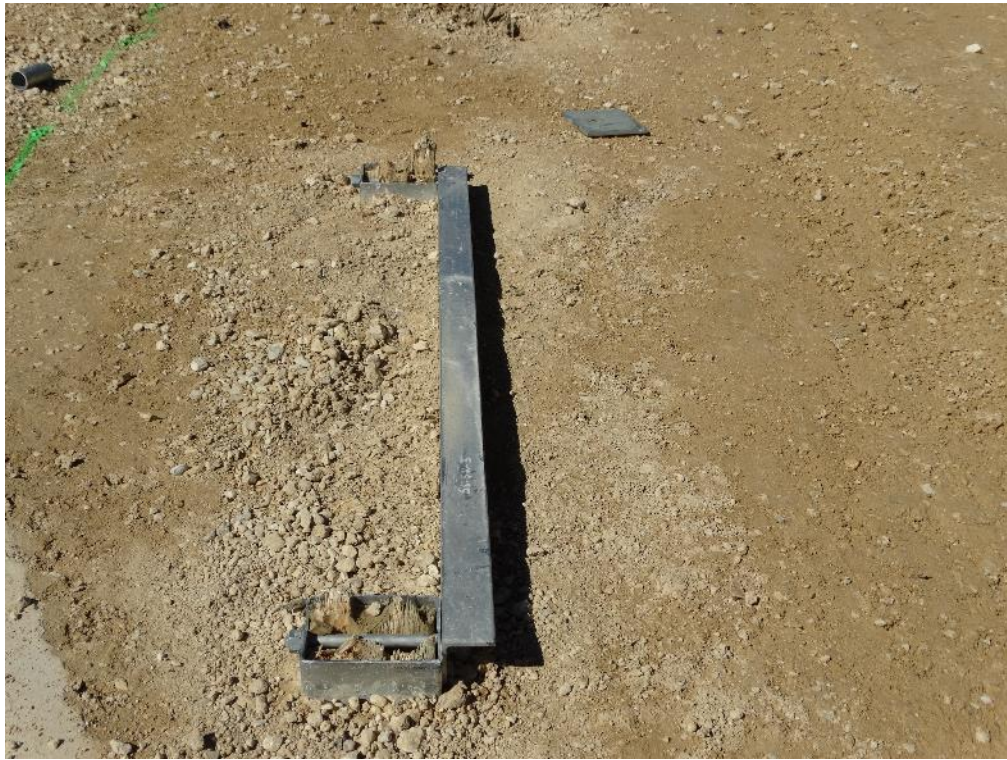
Figure 3.15: Post Test – Foundation Sleeves at Posts 1 and 2
