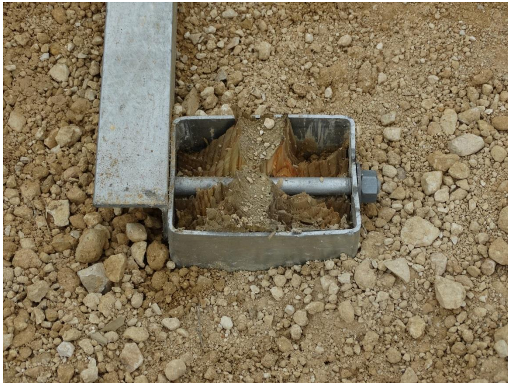
Figure 3.10: Post Test – Foundation Sleeve at Post 2
