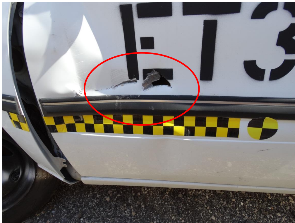
Figure 3.43: Post Test Vehicle – Tear in Door Skin (see Figure 3.3)
