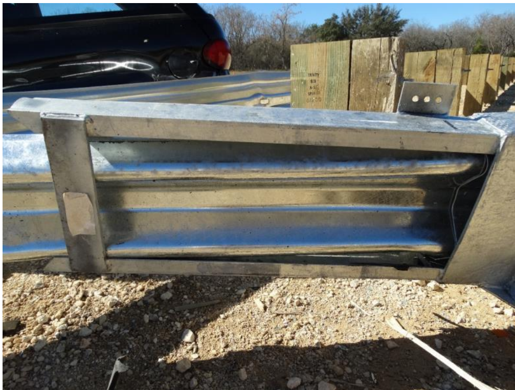
Figure 3.32: Post Test – Traffic Side View of Guide Channels
