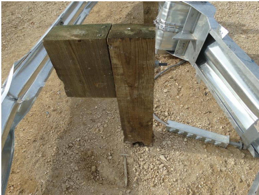
Figure 3.20: Post Test – Side View of Post 5 and Anchor Cable
