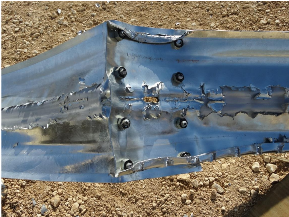
Figure 3.25: Post Test – Extruded Guardrail Splice from between Posts 5 & 6 (Splice Nuts Painted Pre-Test for Visibility in Video)
