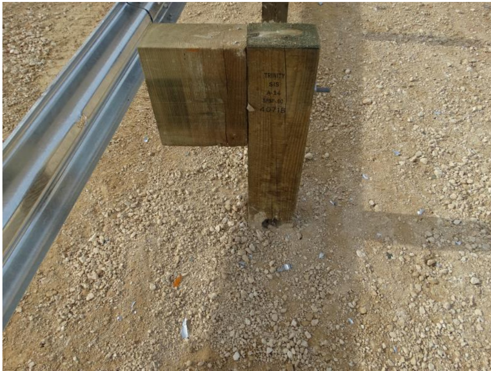
Figure 3.25: Post Test – Side View of Post 7
