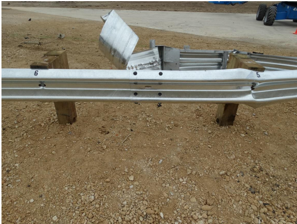
Figure 3.16: Post Test – Splice between Posts 5 & 6 (Splice Bolts Painted Black for Visibility)
