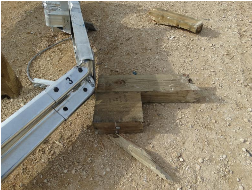
Figure 3.16: Post Test – Traffic Side View of First Splice (Bolts Painted for Visibility in Video)
