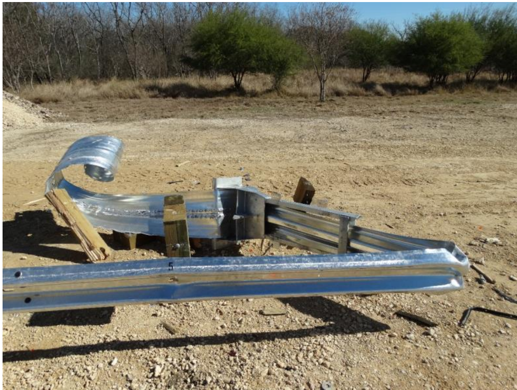
Figure 3.43: Post Test – Traffic Side View of Gated End Terminal
