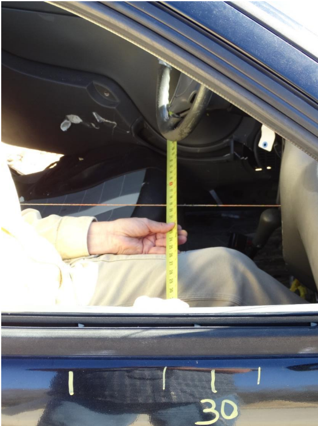
Figure 3.81: Measuring Interior Deformation
