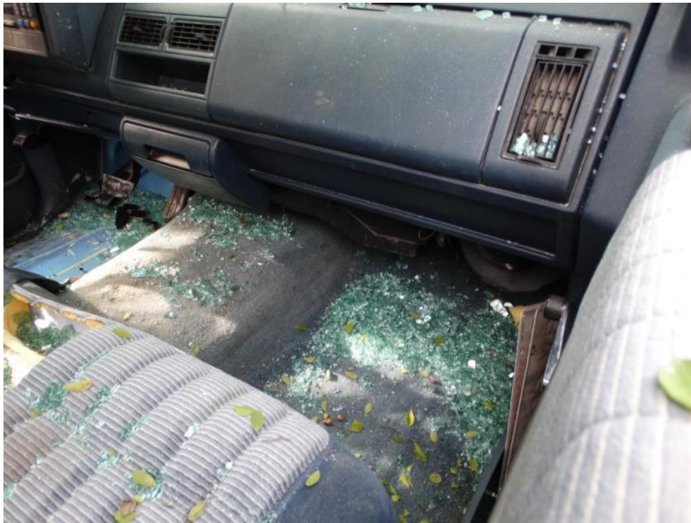
Figure 3.59: Post-Test – Passenger Side Floorboard (Damage due to Impact with Tree)
