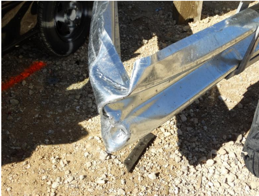
Figure 3.29: Post Test – Traffic Side View of Folded W Beam at Post 4
