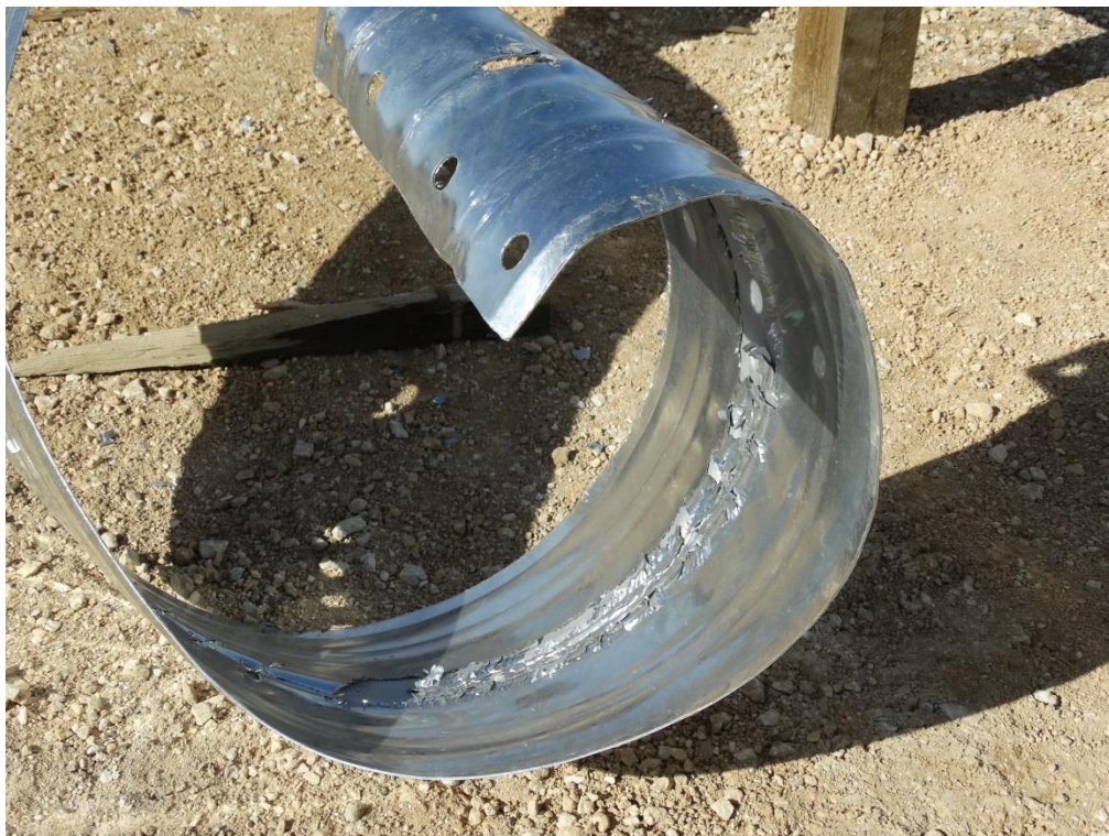
Figure 3.21: Post Test – Extruded Guardrail Coil
