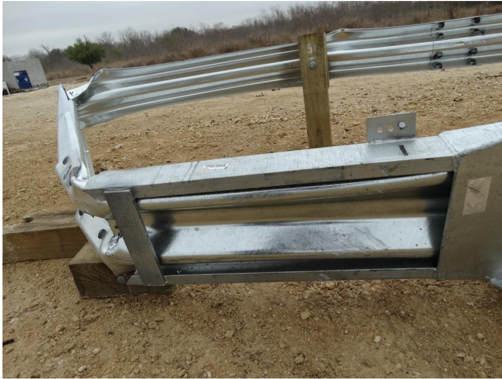
Figure 3.26: Post Test – Traffic Side of Guide Channels
