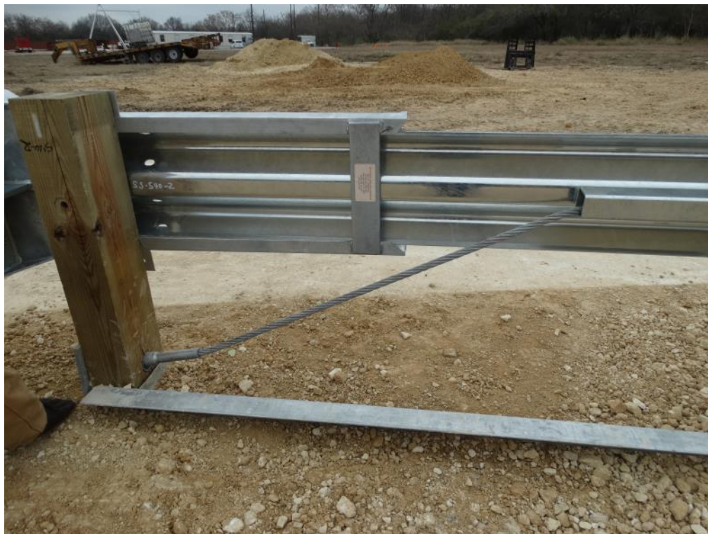
Figure 2.8: ET Plus Head and Anchor Cable Assembly
