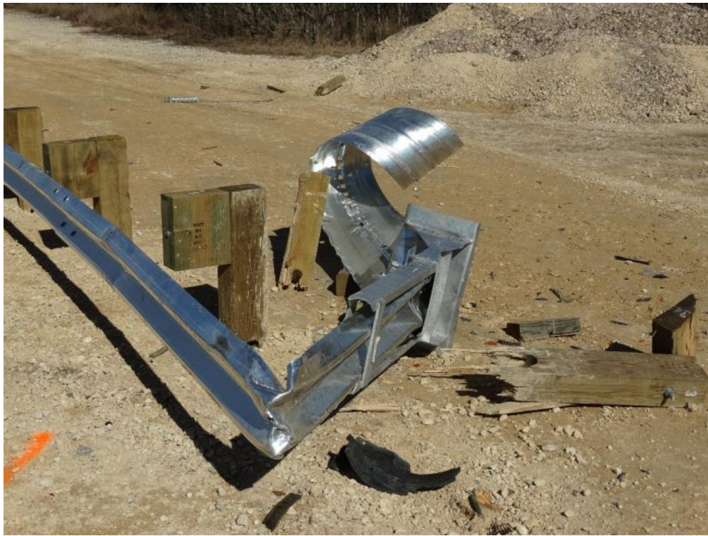
Figure 3.44: Post Test – Traffic Side View of Gated End Terminal
