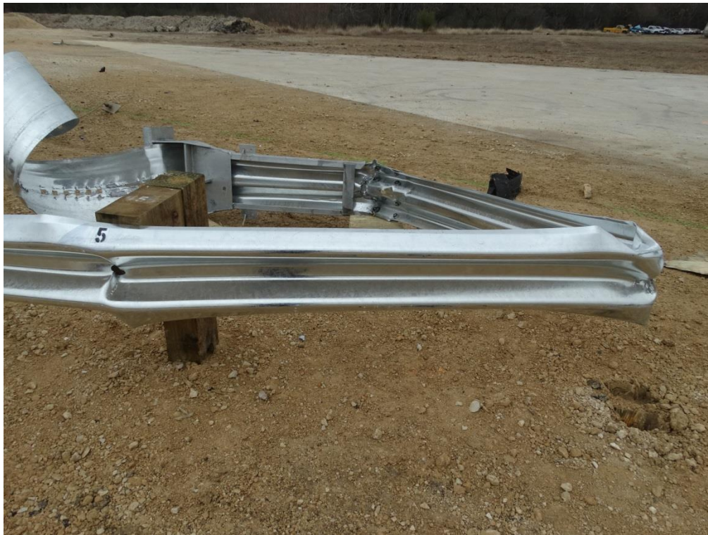
Figure 3.18: Post Test – Gated Guardrail, View from Traffic Side
