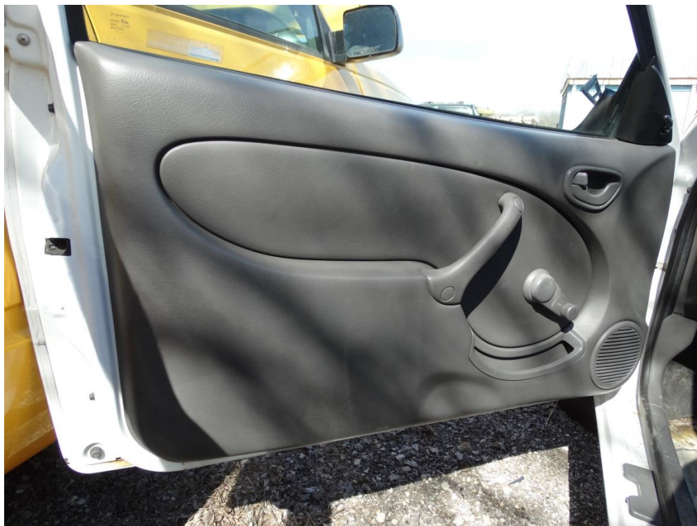
Figure 3.44: Post Test Vehicle – Door Panel Intact behind Exterior Tear
