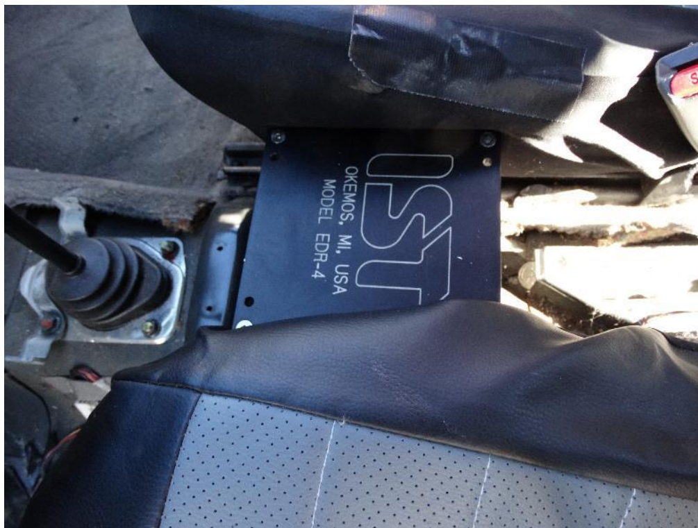
Figure 2.27: EDR Mounted in Test Vehicle for Test ET31-30
