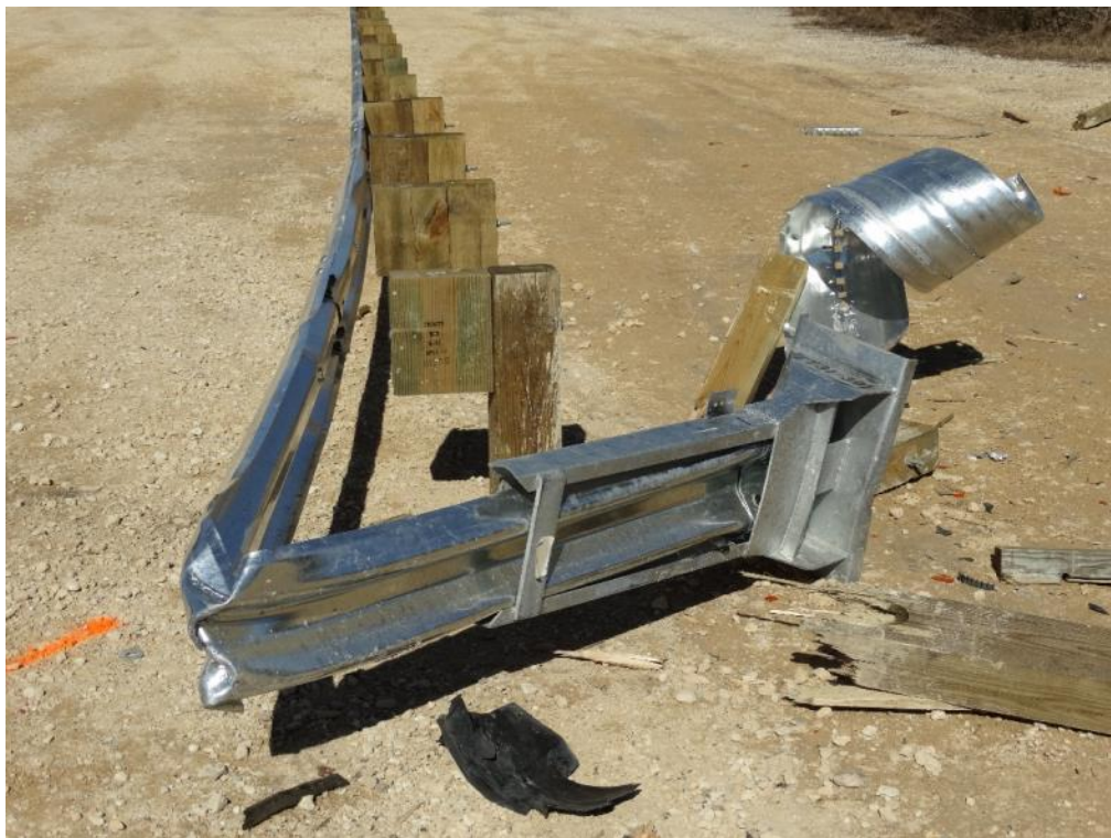
Figure 3.45: Post Test – Traffic Side View of Gated End Terminal
