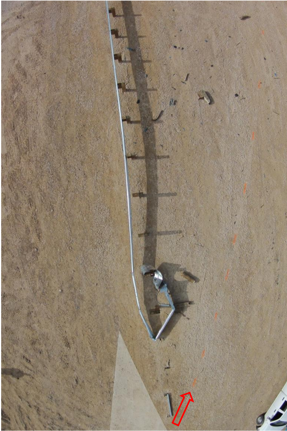
Figure 3.6: Post Test – Debris Field on Non-Traffic Side and Vehicle Path (Orange Paint)
