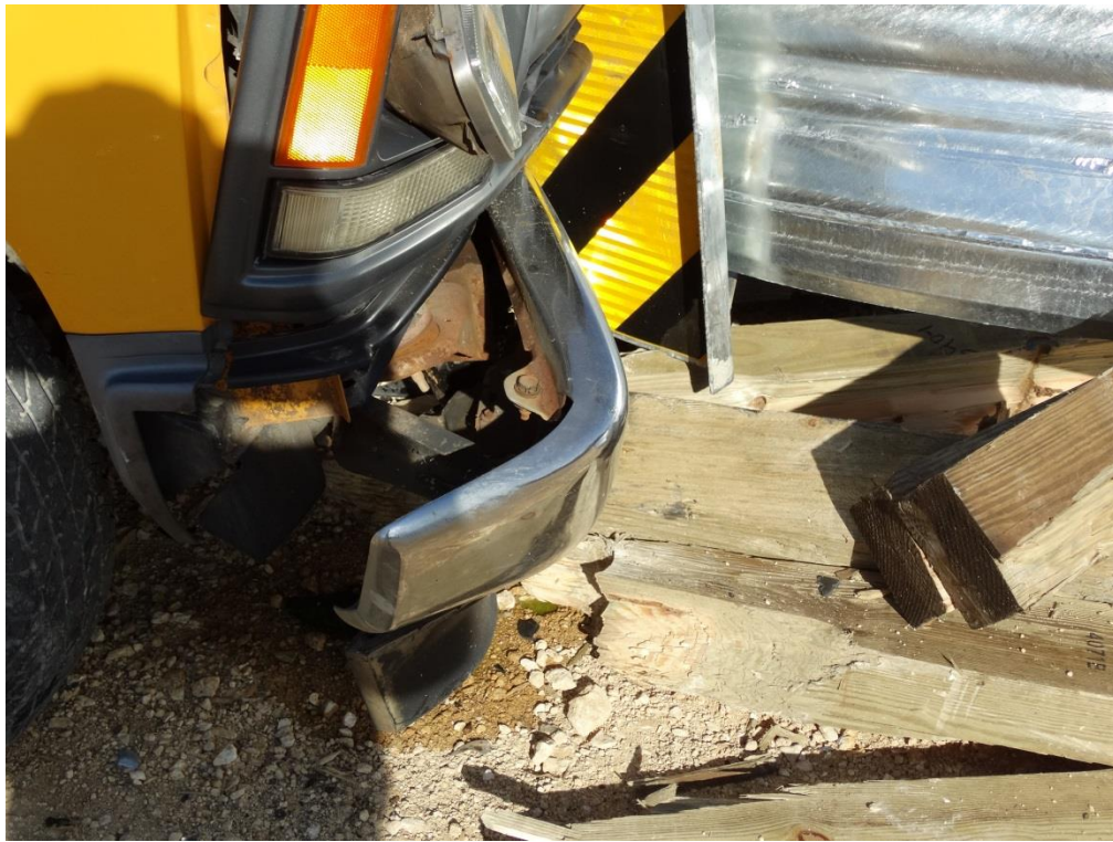
Figure 3.48: Post Test Vehicle – Accumulated Posts at Front of Vehicle
