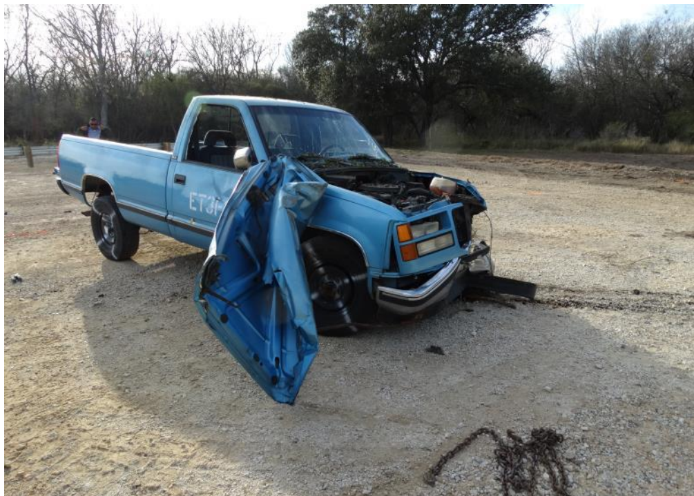
Figure 3.50: Right Side Test Vehicle Damage Following Impact with Tree (Note: Hood Ripped off by Tree Impact)
