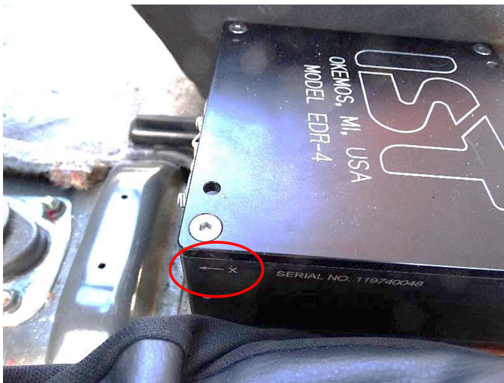
Figure 2.28: Close-up of EDR Orientation as Mounted in Vehicle
