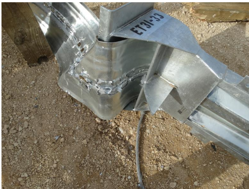
Figure 3.30: Post Test – ET Plus Head and Extruded Rail, Non-Traffic Side
