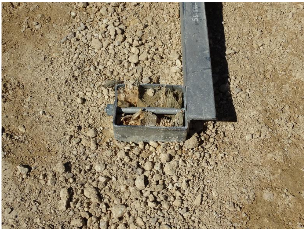
Figure 3.16: Post Test – Foundation Sleeve at Post 1
