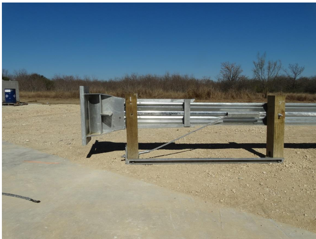
Figure 2.8: ET Plus Head and Anchor Cable Assembly
