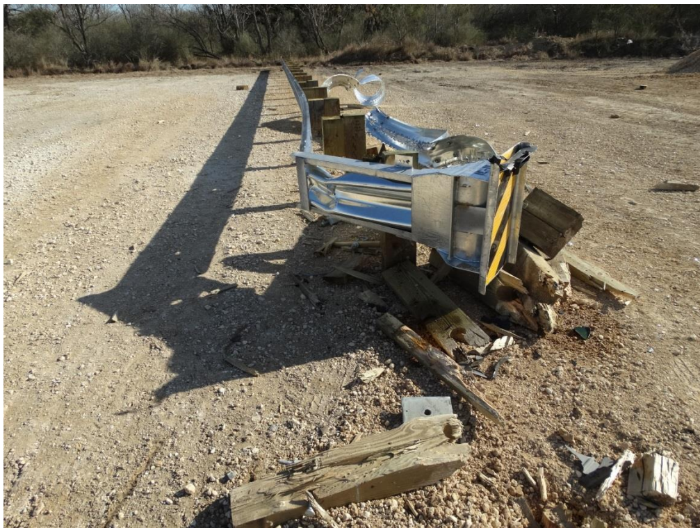
Figure 3.37: Post-Impact Test Article after Vehicle Removed
