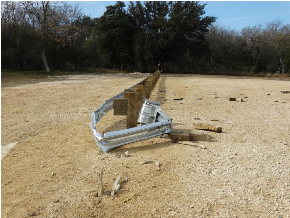
Figure 3.35: Post Test – Debris Field on Non-Traffic Side
