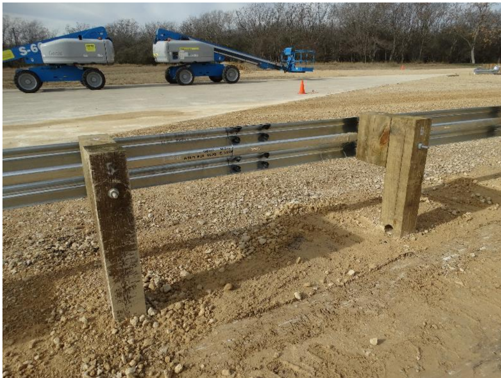
Figure 2.14: Second Guardrail Panel Splice Joint Mid-Span between Posts 5 & 6 – Non-Traffic Side (Nuts Painted for Visibility in Video)
