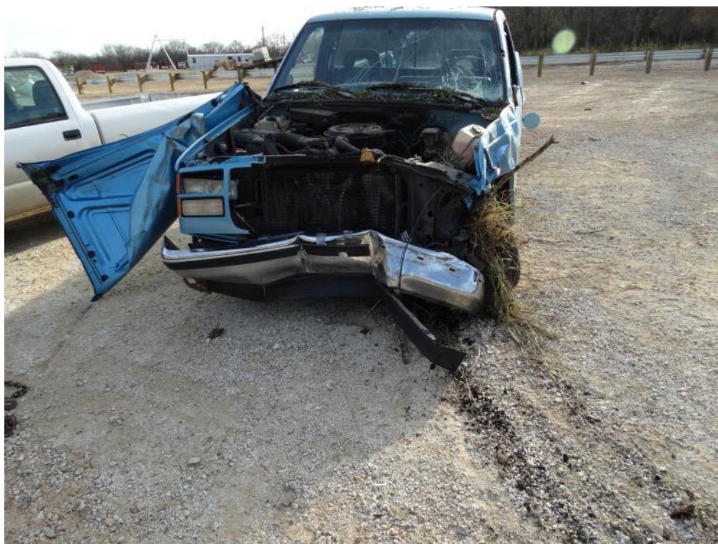
Figure 3.48: Test Vehicle Damage due to Impact with Tree
