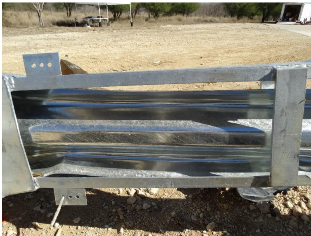
Figure 3.41: Post Test – Non-Traffic Side View of Guide Channels
