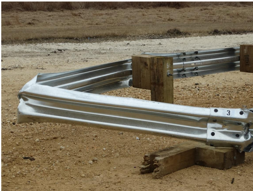
Figure 3.19: Post Test – Gated Guardrail
