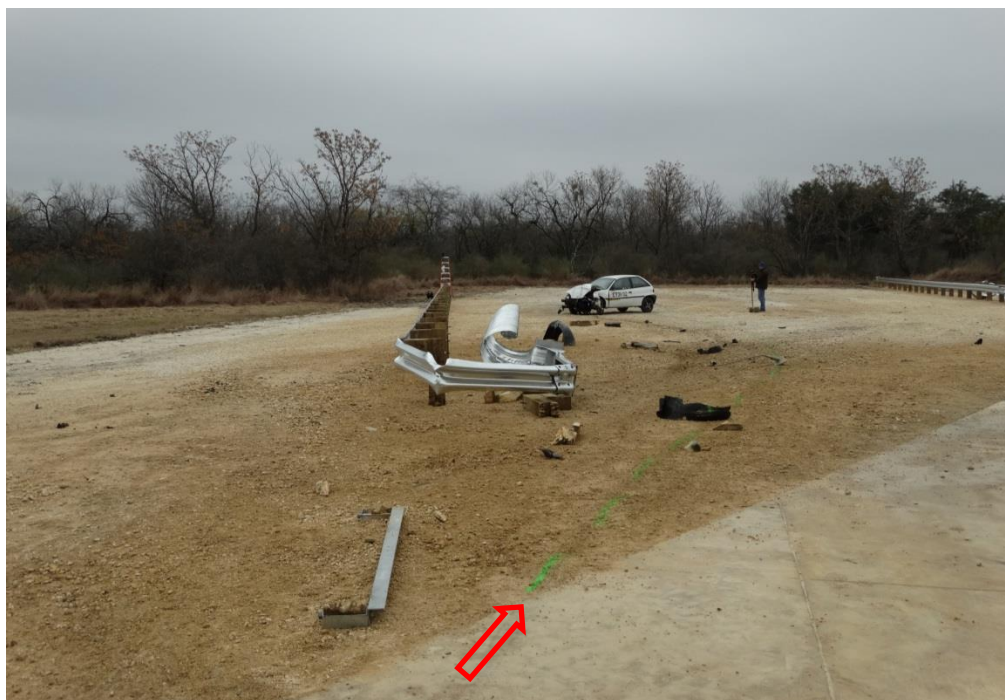
Figure 3.38: Test Vehicle Path of Right Front Tire
