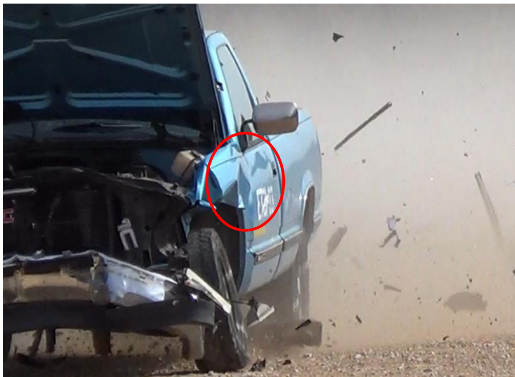
Figure 3.53: Left Side Damage to Vehicle Following ET Plus Impact (see Figure 3.3 at T=0.300seconds)
