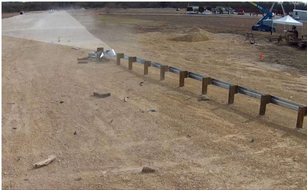
Figure 3.36: Post Test – Debris Field on Non-Traffic Side Viewed from Downstream
