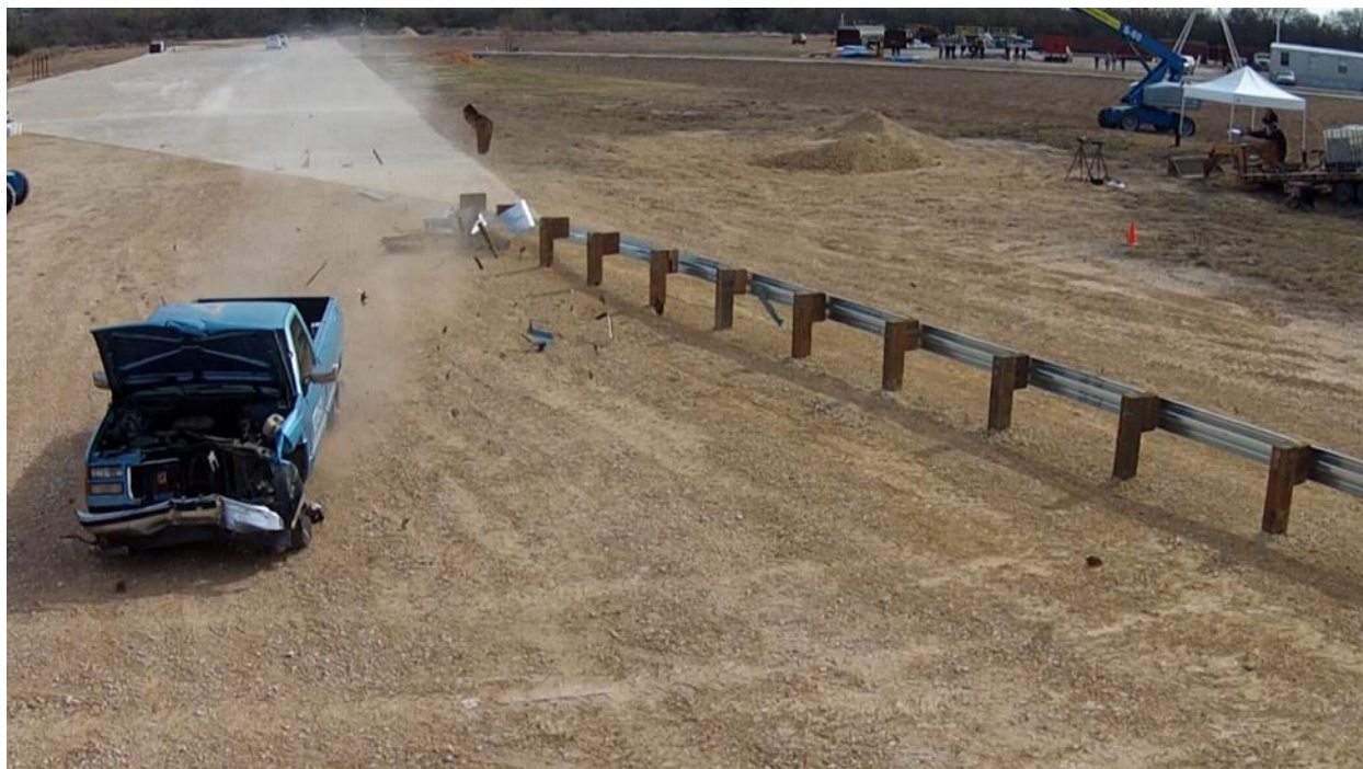
Figure 3.51: Front End Damage to Vehicle Following ET Plus Impact (Drone Camera)
