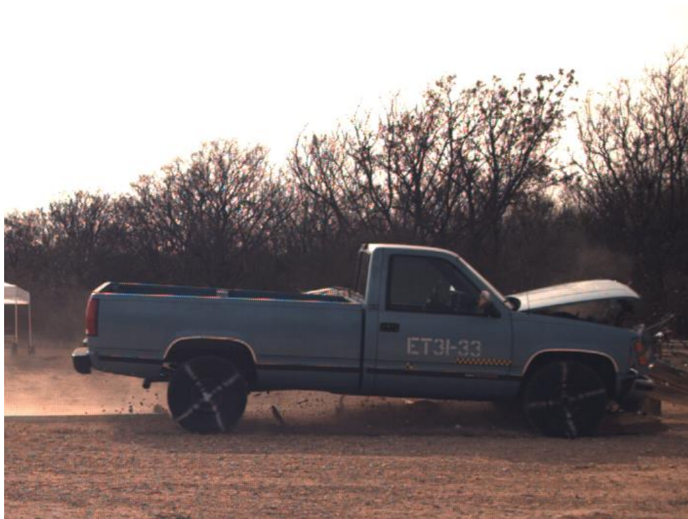
Figure 3.55: Right Side Damage to Vehicle Following ET Plus Impact
