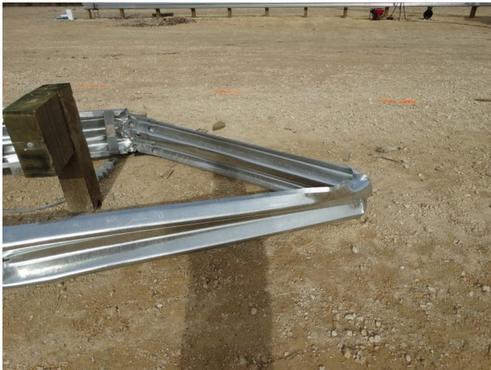
Figure 3.18: Post Test – Traffic Side View of W Beam Fold at Post 4
