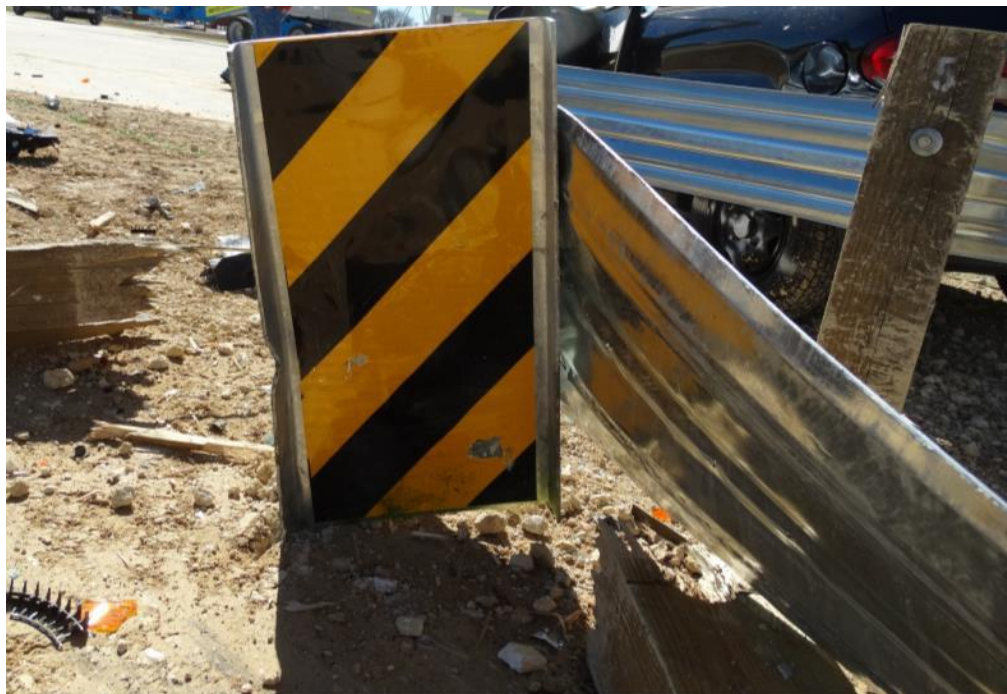
Figure 3.12: Post Test – End View of Impact Plate
