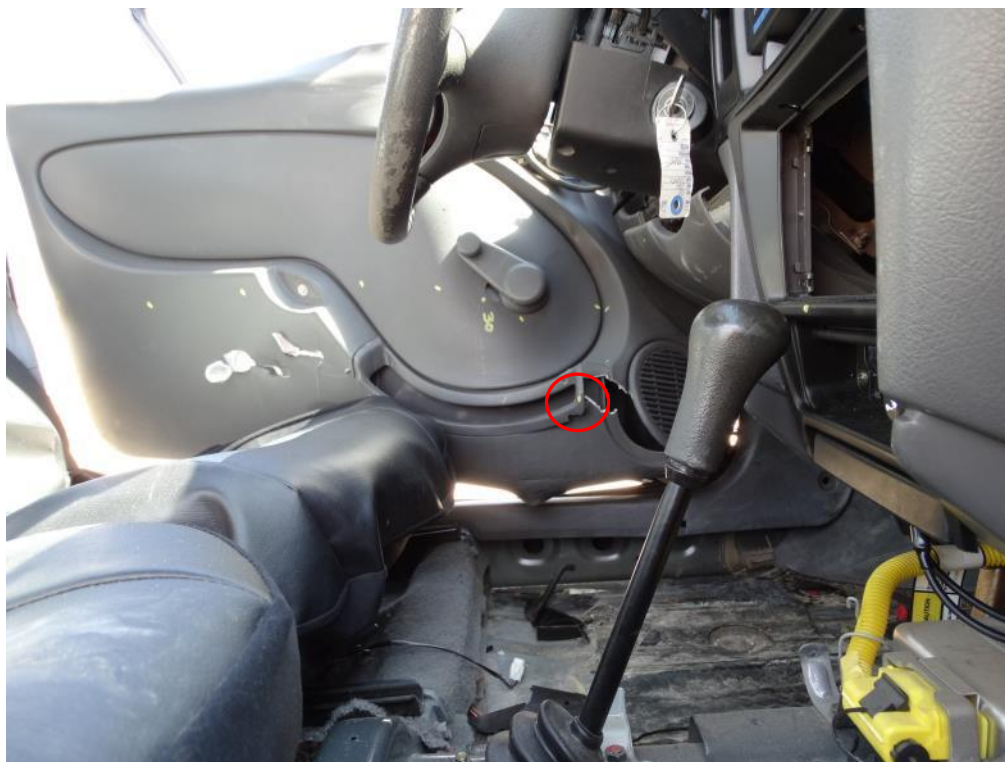
Figure 3.82: Location of Maximum Interior Deformation
