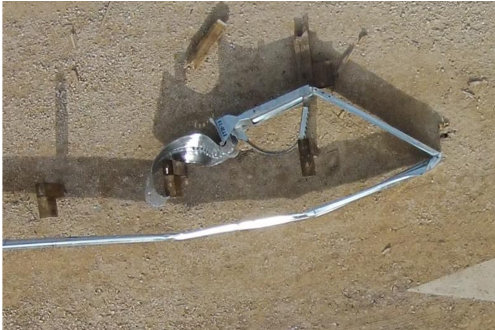
Figure 3.7: Post Test – Overhead View of Gated Terminal
