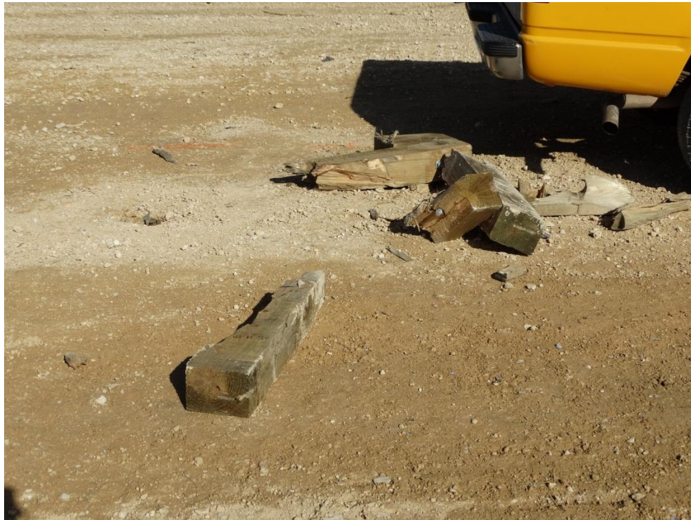
Figure 3.11: Post Test – Posts 1, 2, 3 and 4 at Rear of Truck
