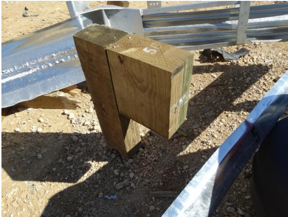
Figure 3.21: Post Test – Traffic View of Post 5 Blockout
