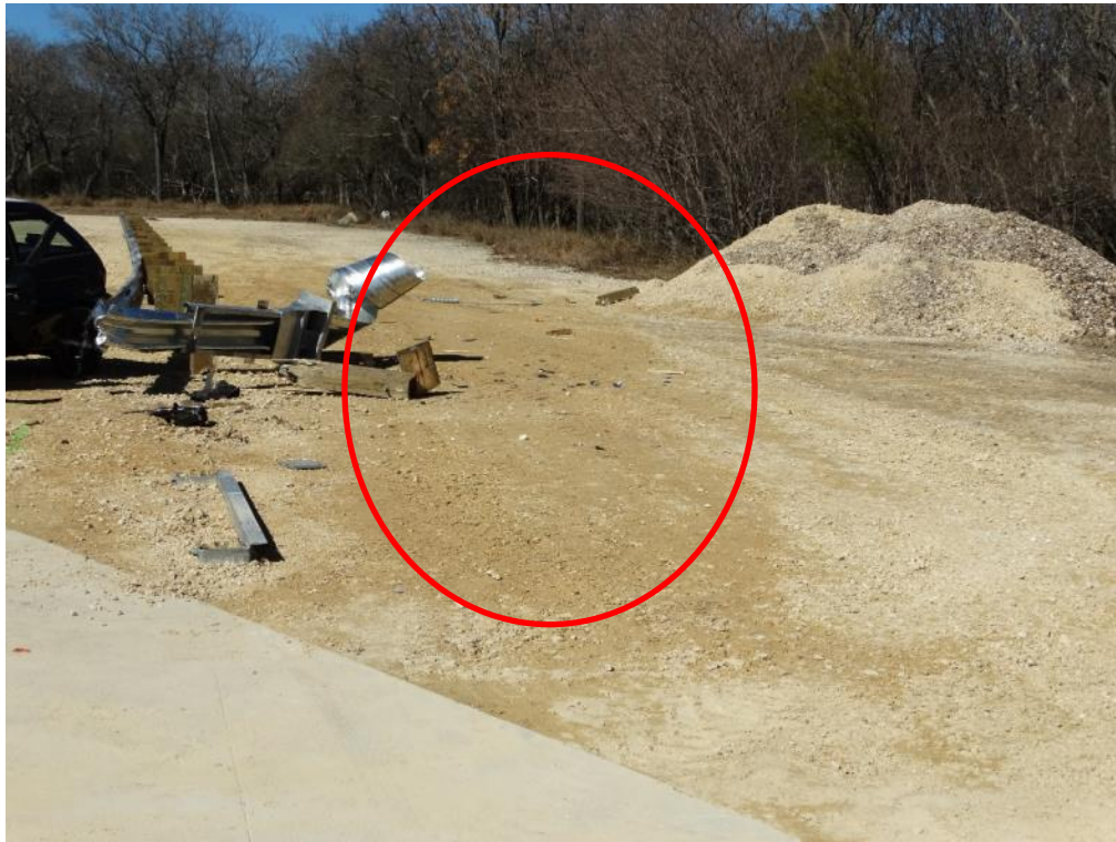
Figure 3.50: Post Test – Debris Field on Non-Traffic Side
