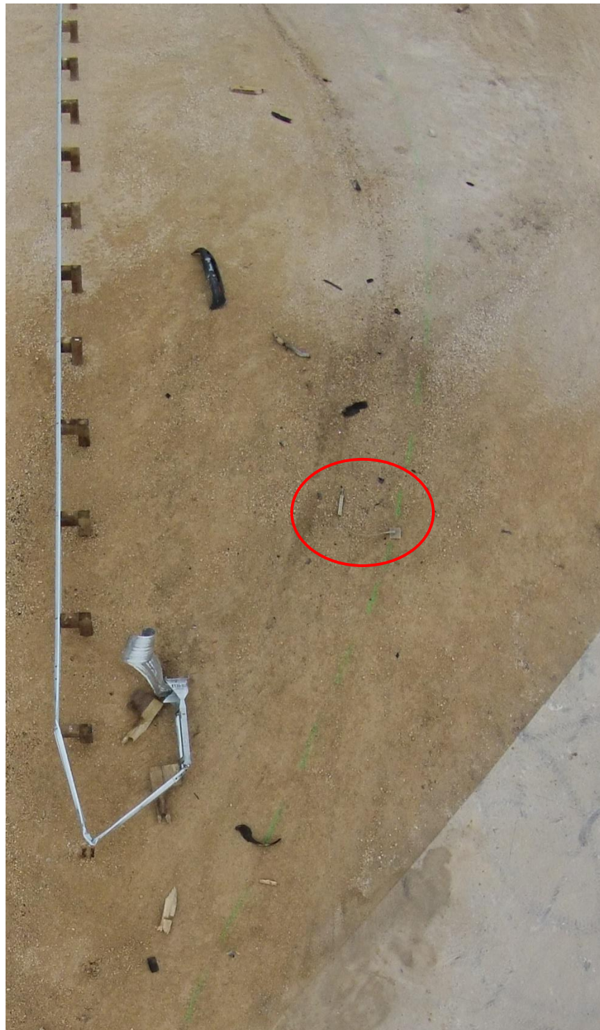
Figure 3.32: Post Test – Debris Field on Non-Traffic Side (Anchor Cable Indicated)
