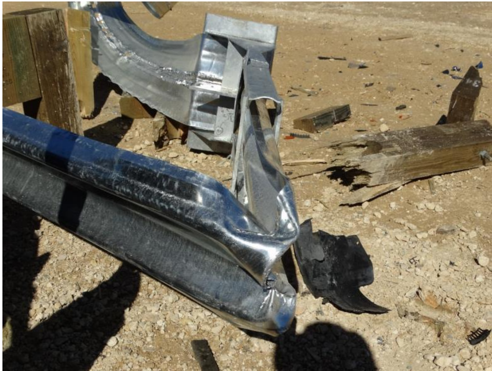
Figure 3.31: Post Test – Upstream View of Guide Channel Entrance
