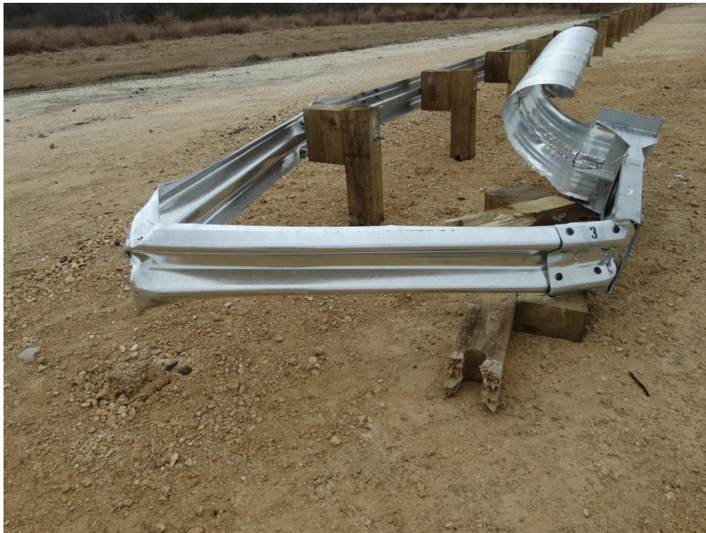
Figure 3.20: Post Test – Gated Guardrail
