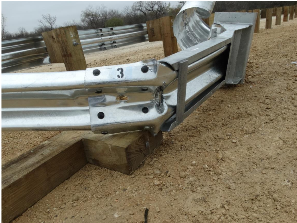
Figure 3.27: Post Test – Traffic Side of Guide Channel Entrance
