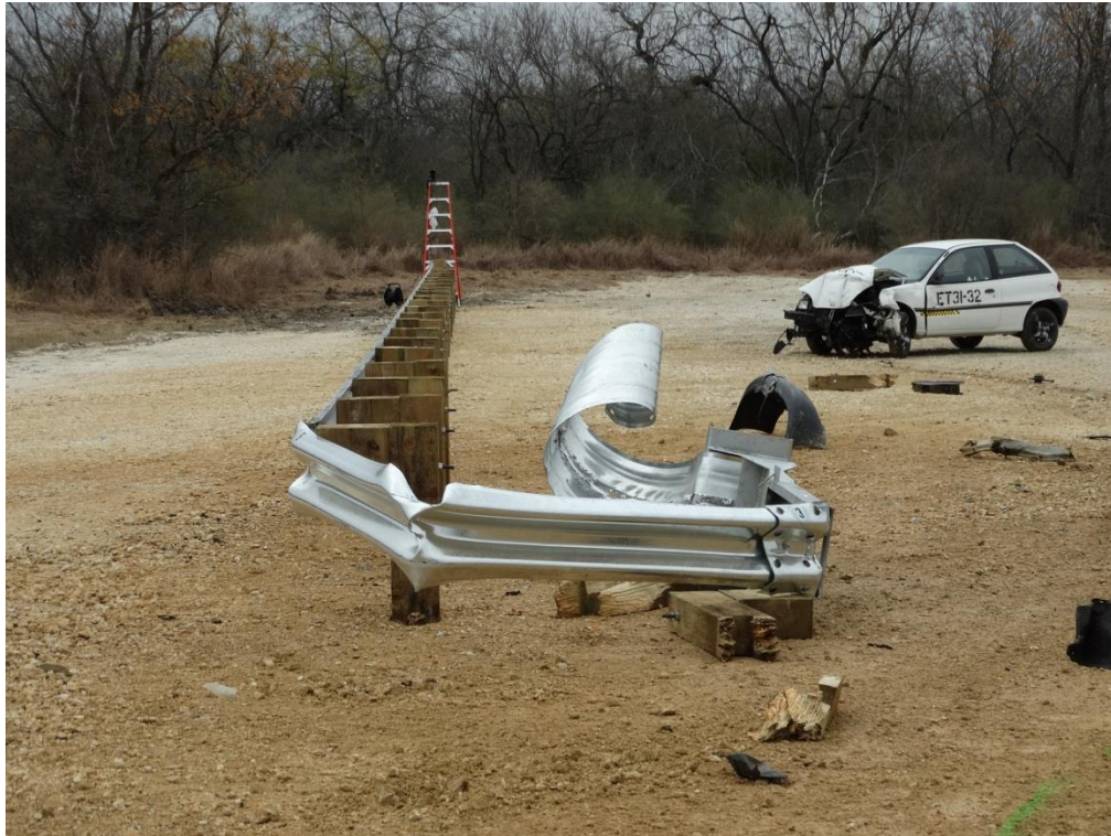
Figure 3.6: Post-Impact Condition of the Test Article and Vehicle
