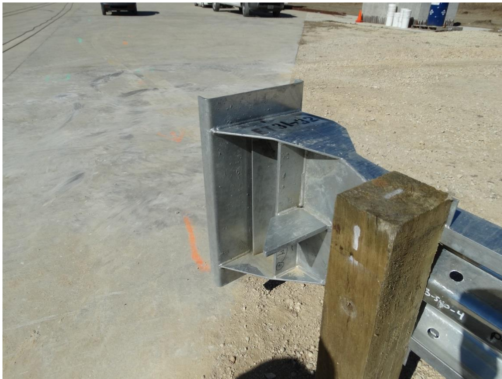
Figure 2.18: ET Plus Head Looking Upstream at Post 1 (see Appendix B for Dimensions)
