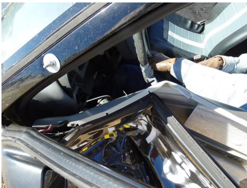
Figure 3.69: Post Test Vehicle – Left Side Door and Door Panel
