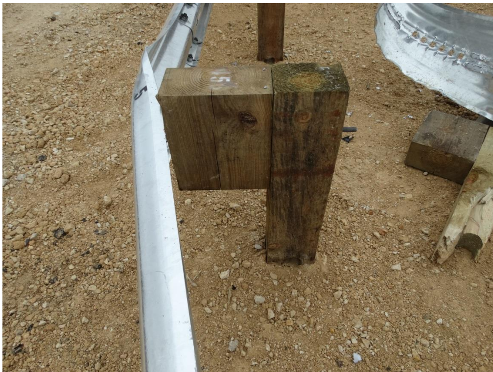
Figure 3.13: Post Test – Post 5, Side View
