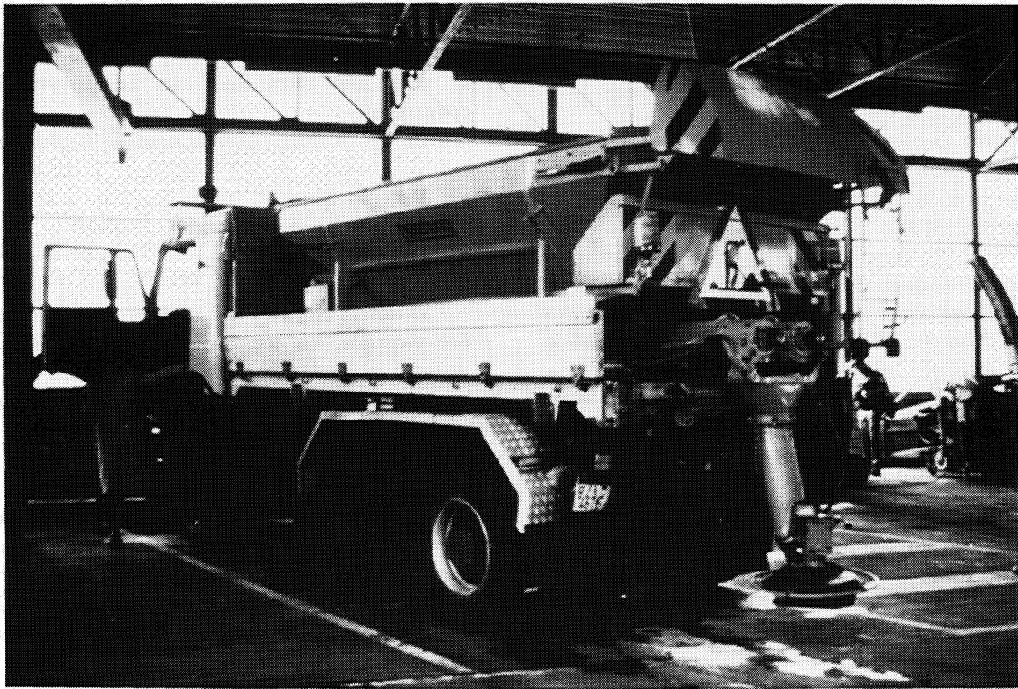
Figure 12. Air foil on rear of salt spreader, Switzerland.
