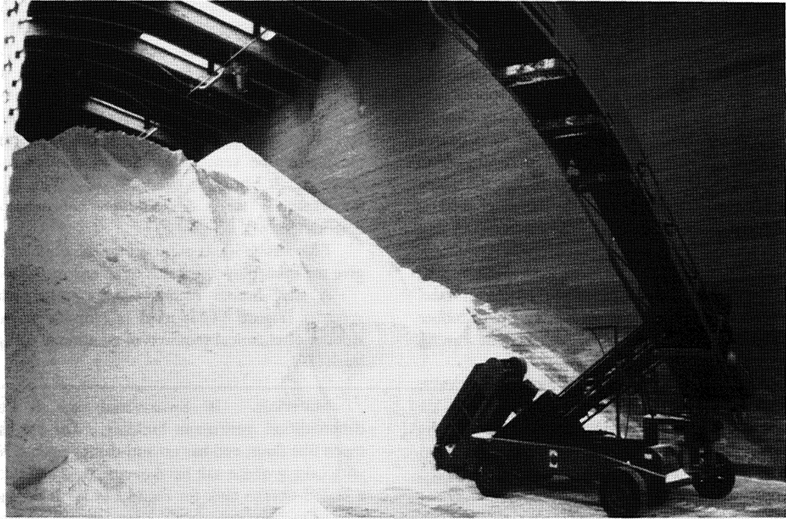
Figure 11. Conveyor Salt Loader in Switzerland.
