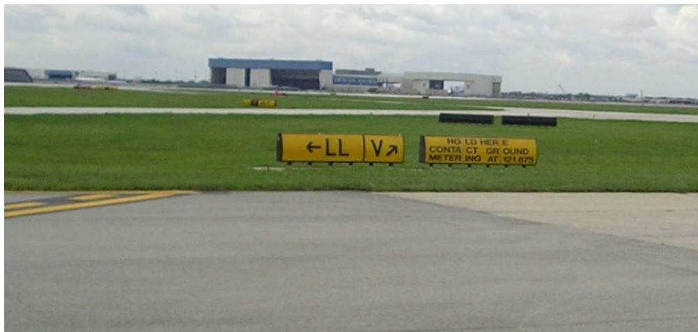
Figure 7. Picture of Ground Signage at Chicago O'Hare Instructing General Aviation Pilots To Hold and Contact Ground Control Before Proceeding
