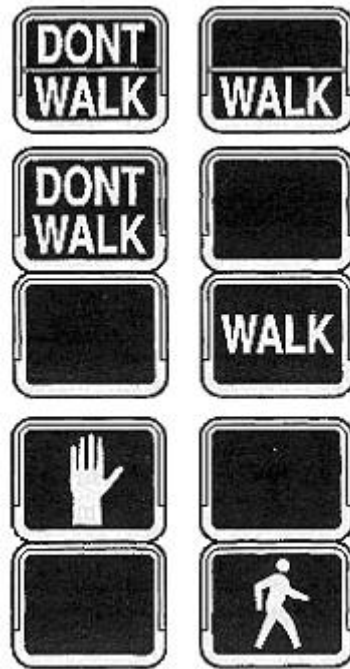
Figure 11-13. Illustration. Pedestrian crossing signals should be clear and understandable by all users.
