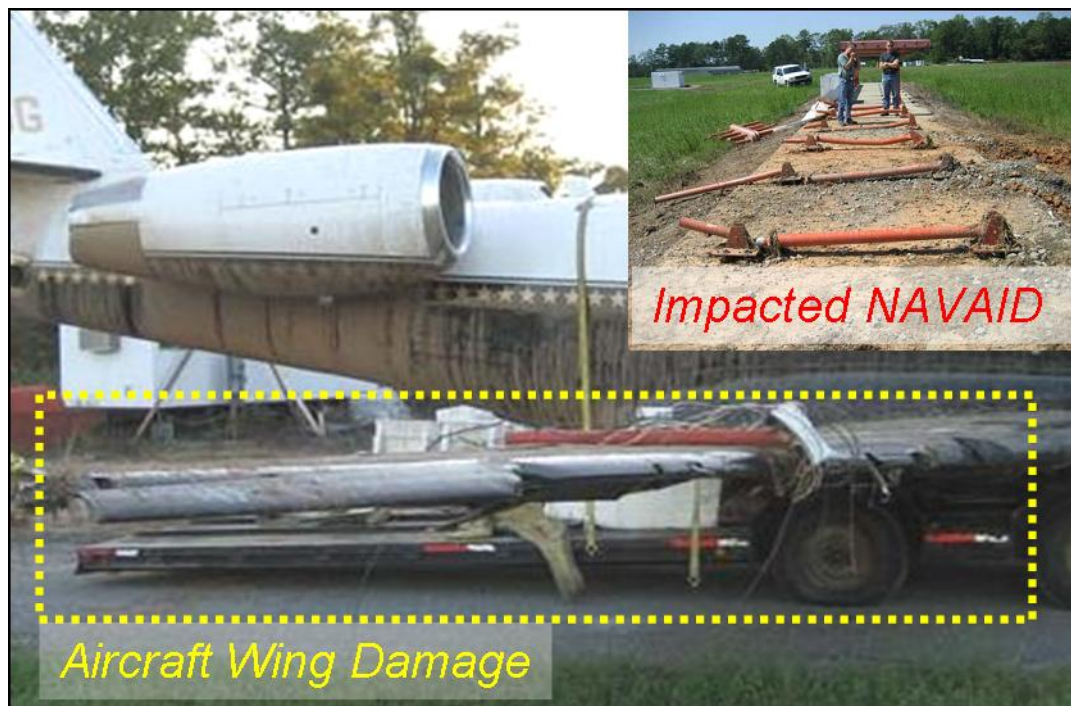
Figure 3. Aircraft Damage from Hitting NAVAID at Dekalb-Peachtree Airport
