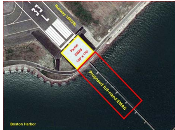
Figure 7. RSA EMAS Extension Project at Boston Airport
