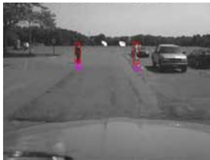
Visual output of the pedestrian-detection system as it recognizes crossing pedestrians.
