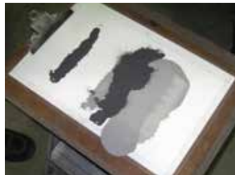
Fly ash with different carbon content levels.
