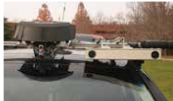
Camera and LIDAR equipment mounted on the roof of the test vehicle.
