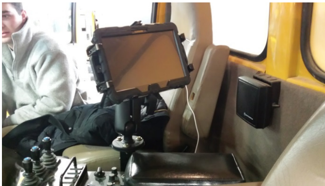
Figure 3-1. Tablet Computer Installed in a WYDOT Plow Truck
