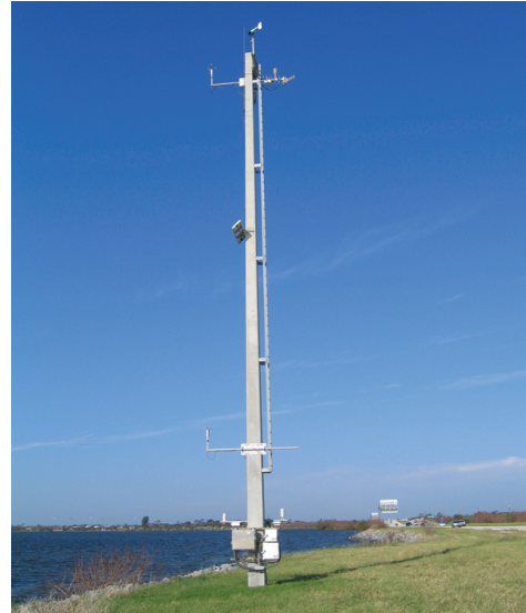
Figure 2. Road Weather Information System (RWIS) Environmental Sensor Station (ESS)
