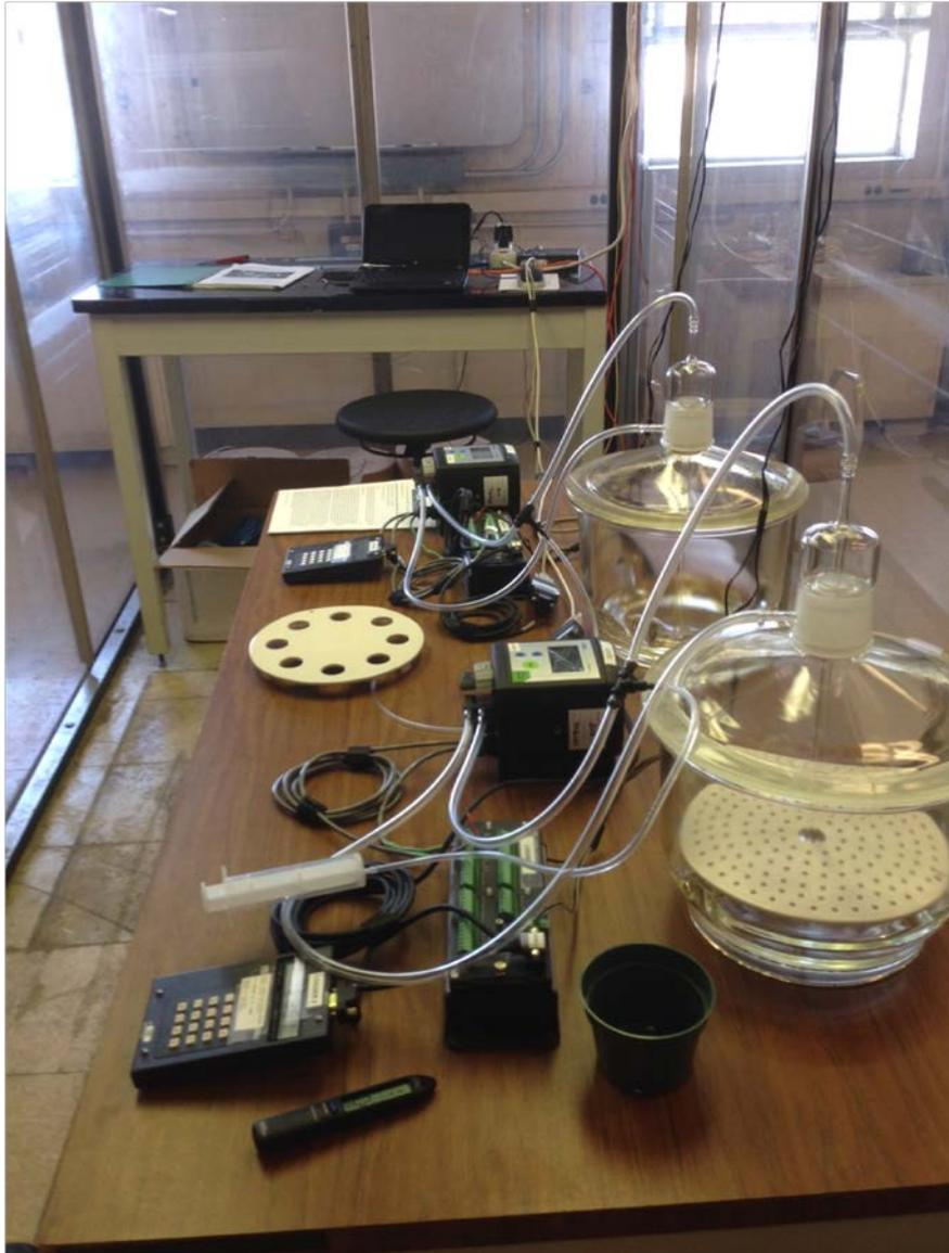
Two identical set-ups including glass chamber, Draeger chemical sensor, tubing, and syringe for injection of gas.
