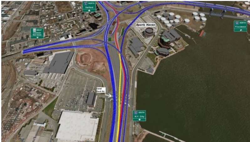
Figure 2: This 4D model communicates traffic staging and necessarily includes the whole project. 2
