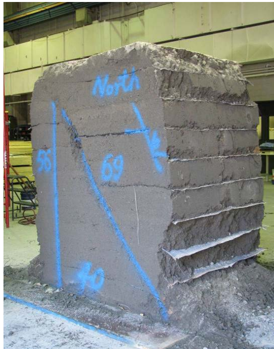
Figure 191. Photo. Back view of failure planes of the composite mass after test 5.
