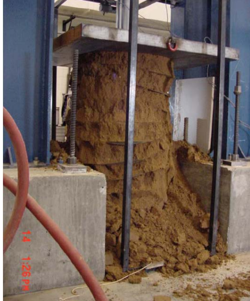
Figure 15. Photo. Unconfined test specimen after testing. (31)
