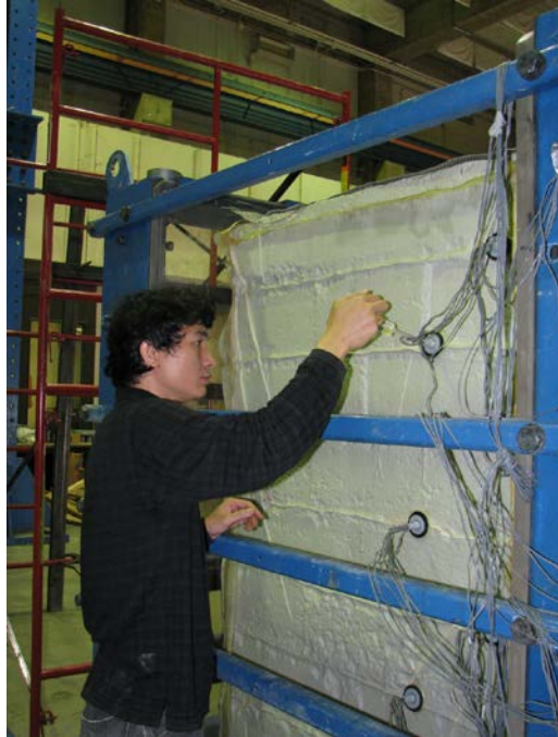
Figure 137. Photo. Sealing the connection between cable and membrane with epoxy to prevent air leaks.
