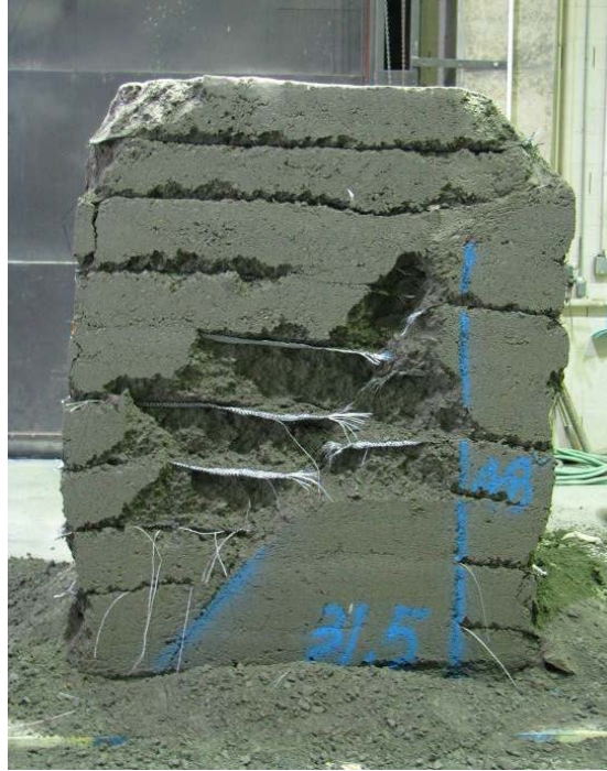
Figure 190. Photo. Front view of failure planes of the composite mass after test 5.
