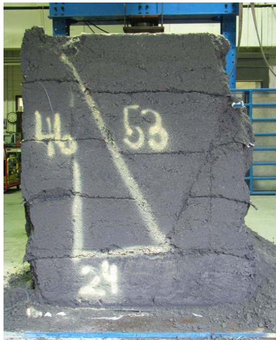
Figure 178. Photo. Back view of failure planes of the composite mass after test 4.
