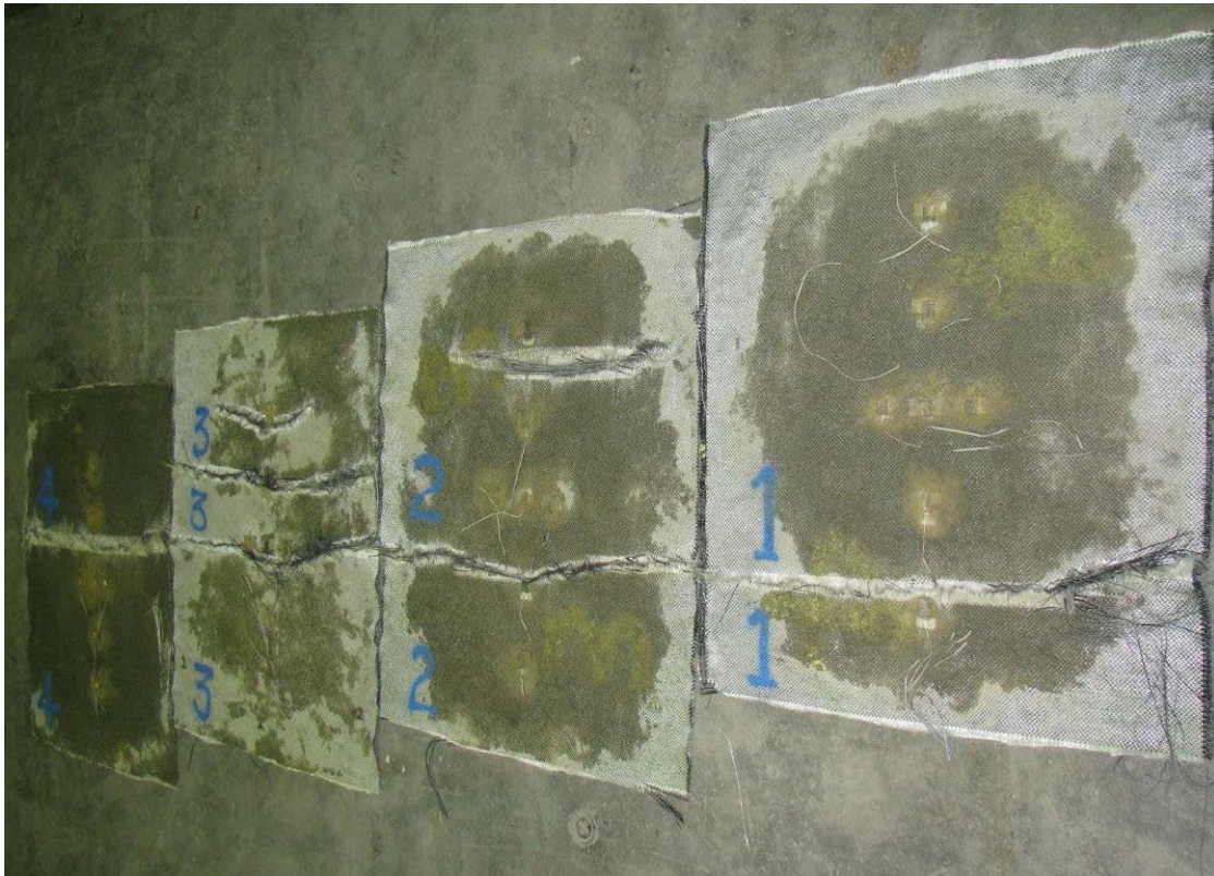
Figure 187. Photo. Aerial view of the reinforcement sheets exhumed from the composite mass after test 4 (numbers indicate sheet number).
