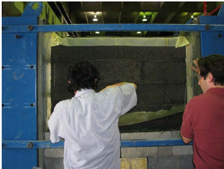
Figure 134. Photo. Removing facing blocks and trimming off excess geosynthetic reinforcement.
