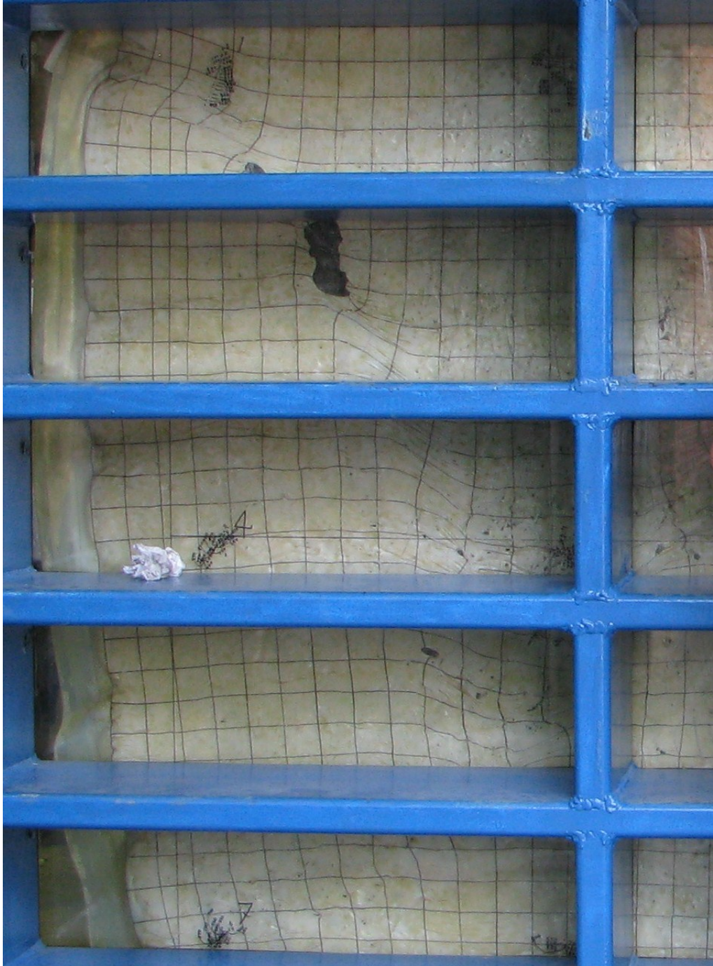
Figure 148. Photo. Close-up of shear bands at failure of area A in figure 147.
