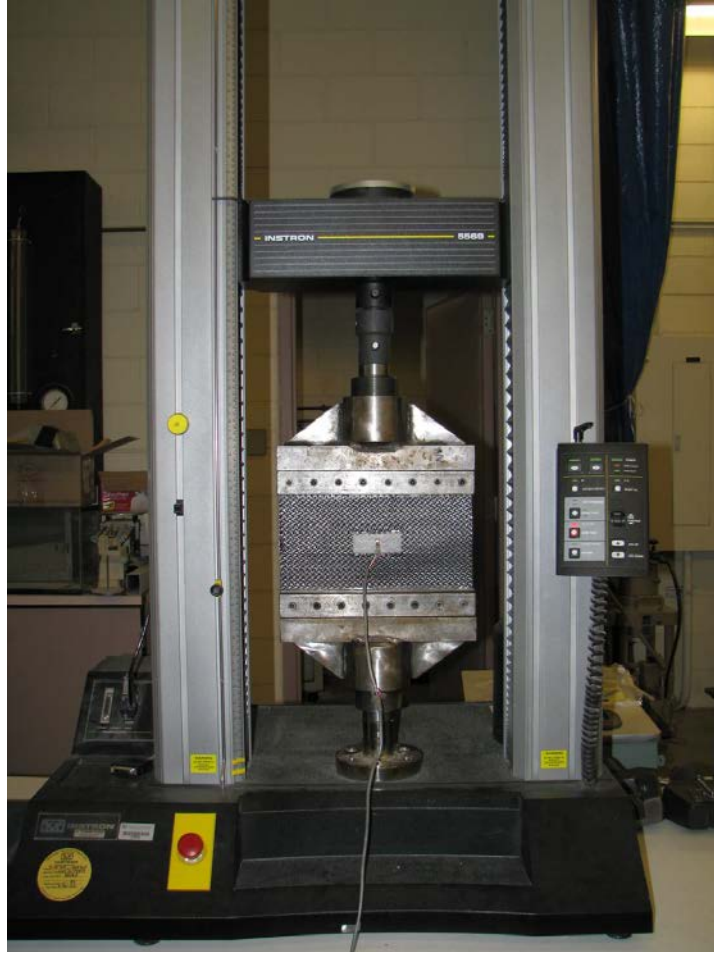
Figure 117. Photo. Uniaxial tension test of Geotex ® 4×4.
