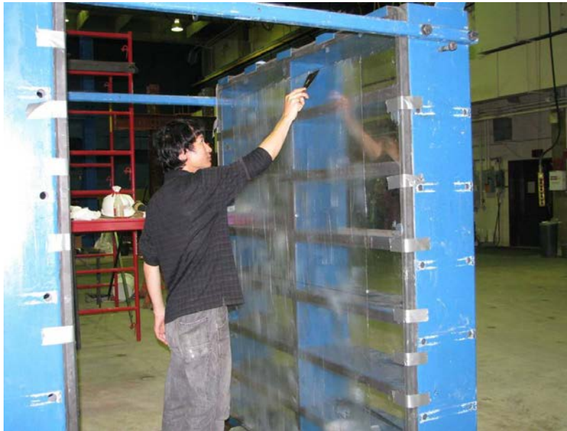
Figure 125. Photo. Applying grease on Plexiglas ® surfaces.
