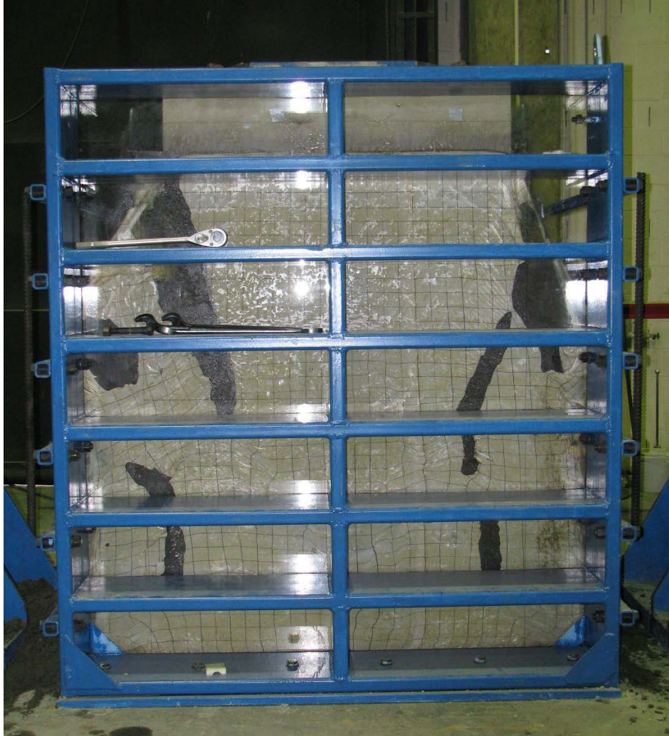
Figure 142. Photo. Soil mass at failure of test 1.
