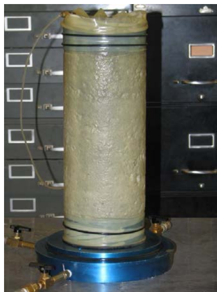
Figure 112. Photo. Typical triaxial test specimen before test.
