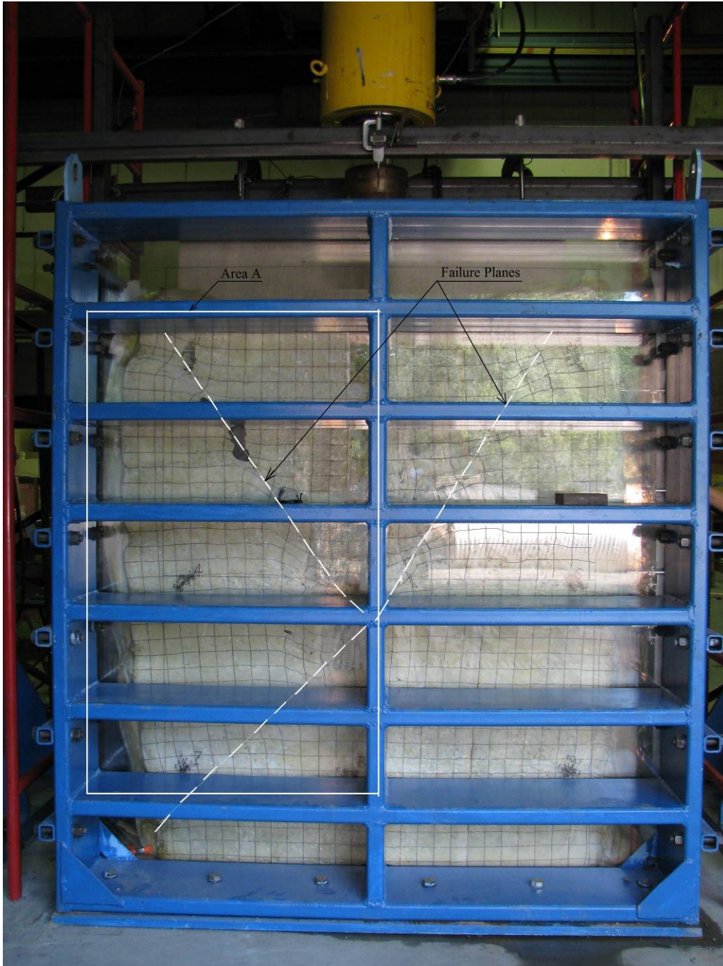
Figure 147. Photo. Composite mass at failure of test 2.
