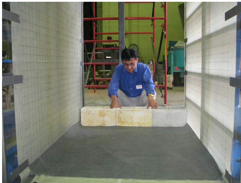
Figure 127. Photo. Placement of the first course of facing block.
