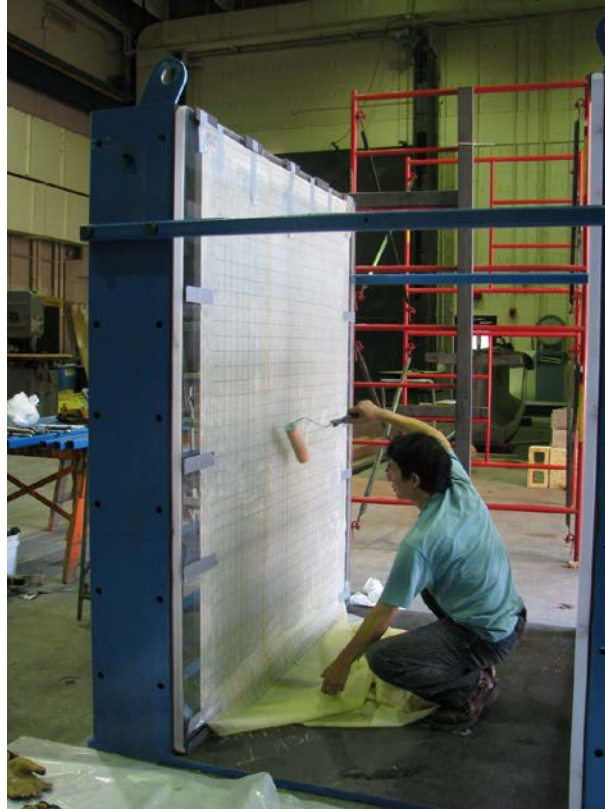
Figure 126. Photo. Attaching membrane.
