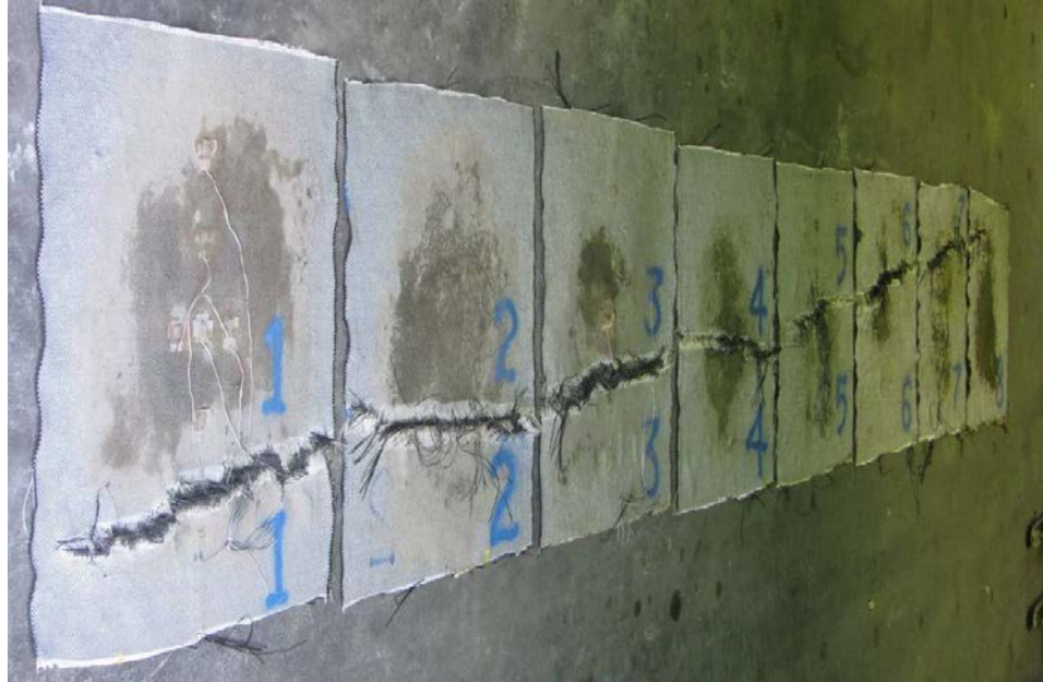
Figure 199. Photo. Aerial view of the reinforcement sheets exhumed from the composite mass after test 5 (numbers indicate sheet number).
