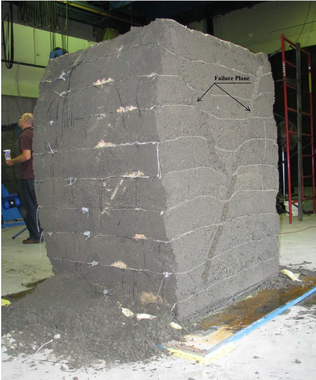
Figure 149. Photo. Failure planes of the composite mass after testing in test 2.
