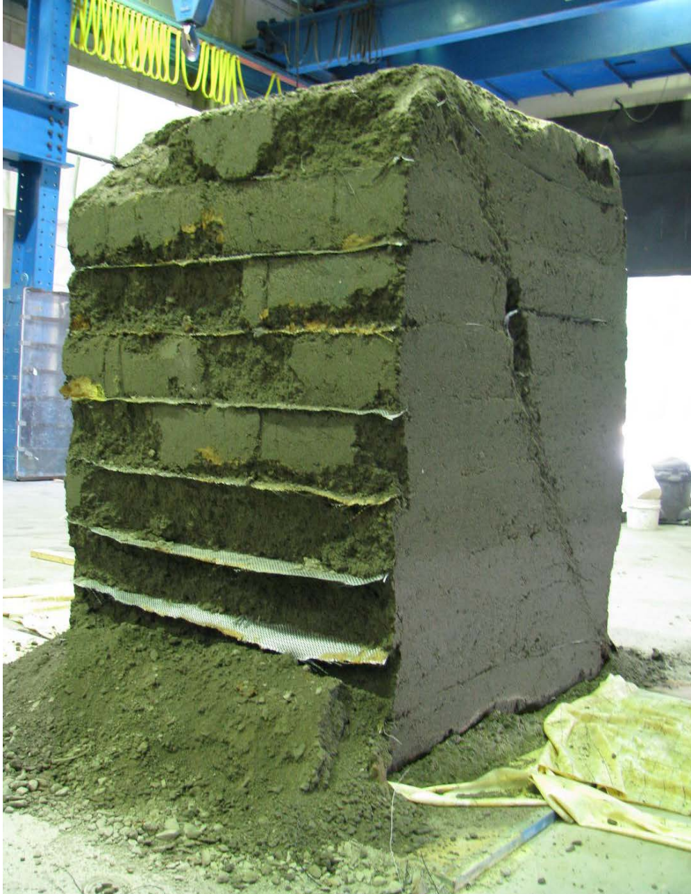
Figure 189. Photo. Composite mass at failure of test 5.
