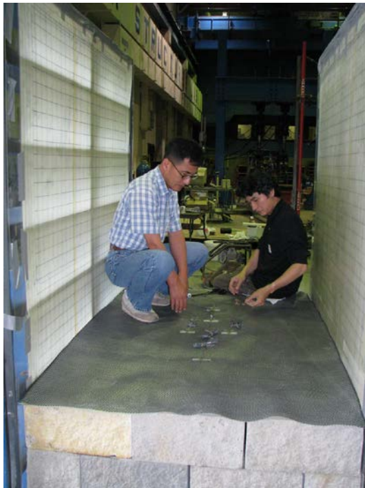
Figure 130. Photo. Placing a reinforcement sheet.
