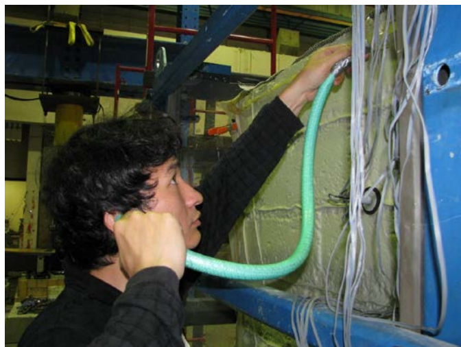
Figure 138. Photo. Checking air leaks under vacuuming.
