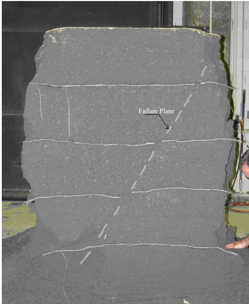
Figure 166. Photo. Composite mass after testing of test 3.
