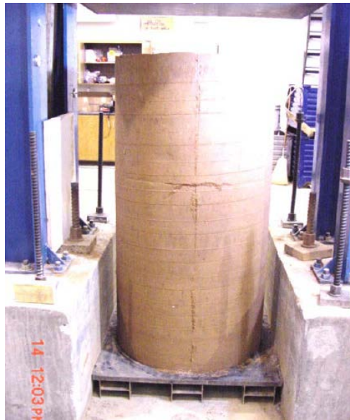
Figure 14. Photo. Unconfined test specimen before testing. (31)
