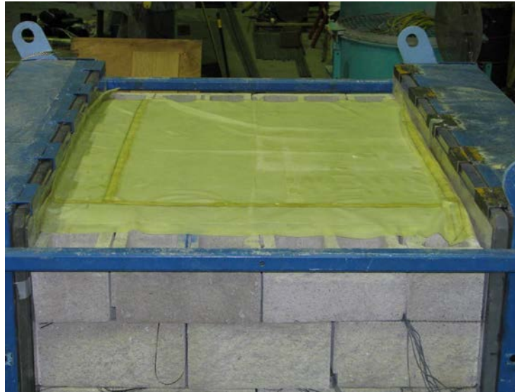
Figure 133. Photo. Top surface of the composite mass covered with a sheet of membrane.
