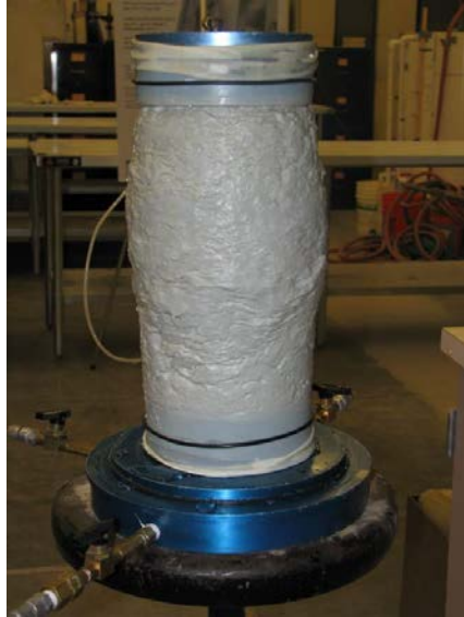
Figure 113. Photo. Typical triaxial test specimen after test.
