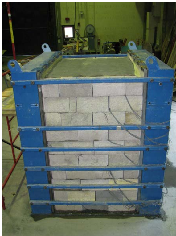
Figure 132. Photo. Completed composite mass with a geotextile sheet on the top surface.
