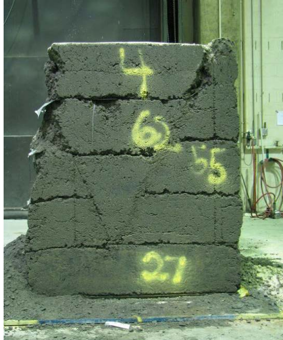
Figure 177. Photo. Front view of failure planes of the composite mass after test 4.
