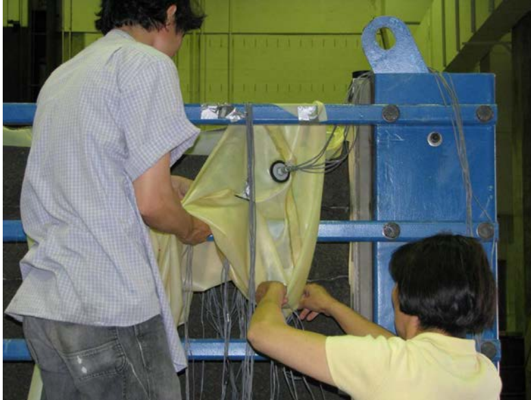
Figure 135. Photo. Inserting strain gauge cables through the membrane sheet.
