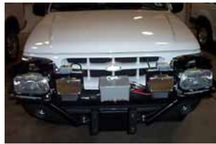
Figure 5. Photo. Hybrid UV-A + halogen low beam.
