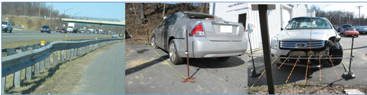
Figure 3. Illustration. NASS CDS data acquisition example showing damaged roadside elements (left, W-beam strong post) and vehicle damage (center, back/left oblique and right, front with measurement rods). (6)
