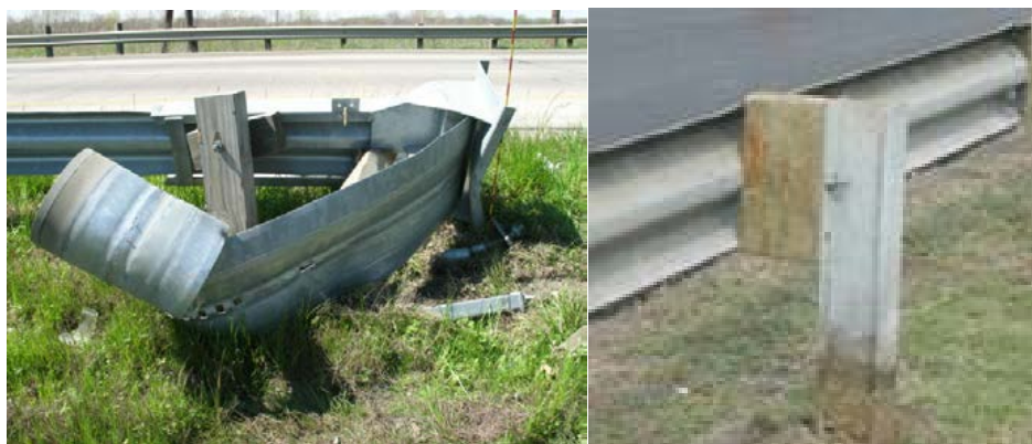
Figure 11. Photo. Case No. 2005049602183 post-crash W-beam strong post (left) contrasted with comparative catalog image (right). (4,14)
