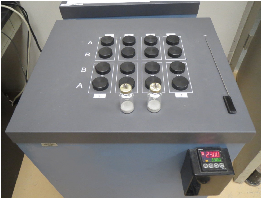
Figure 10. Photo. Isothermal calorimeter and sample specimens via ASTM C1679. (37)
