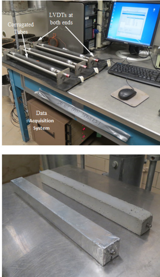
Figure 14. Photo. ASTM C1698 tubes setup (top) and sealed and drying ASTM C157 specimens (bottom). (3,2)
