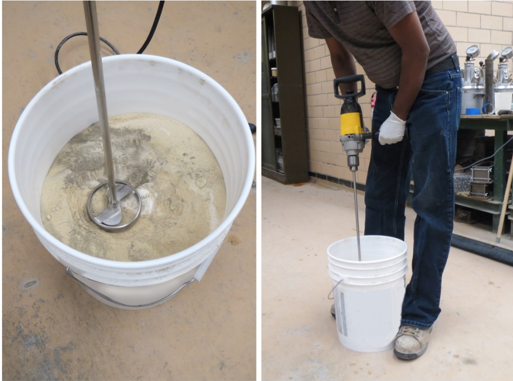
Figure 4. Photo. Mixing M2 grout using a drill and a paddle.
