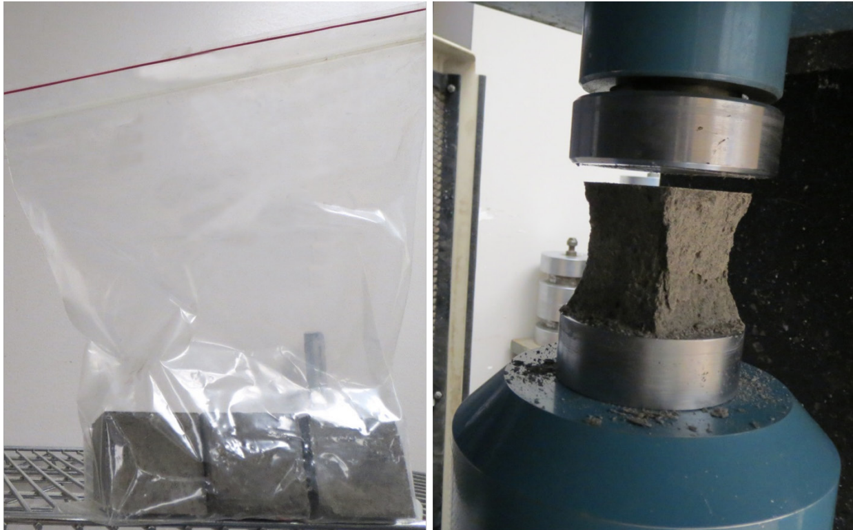
Figure 9. Photo. Compressive strength cube specimens (left) and cube specimen after test via ASTM C109 (right). (36)
